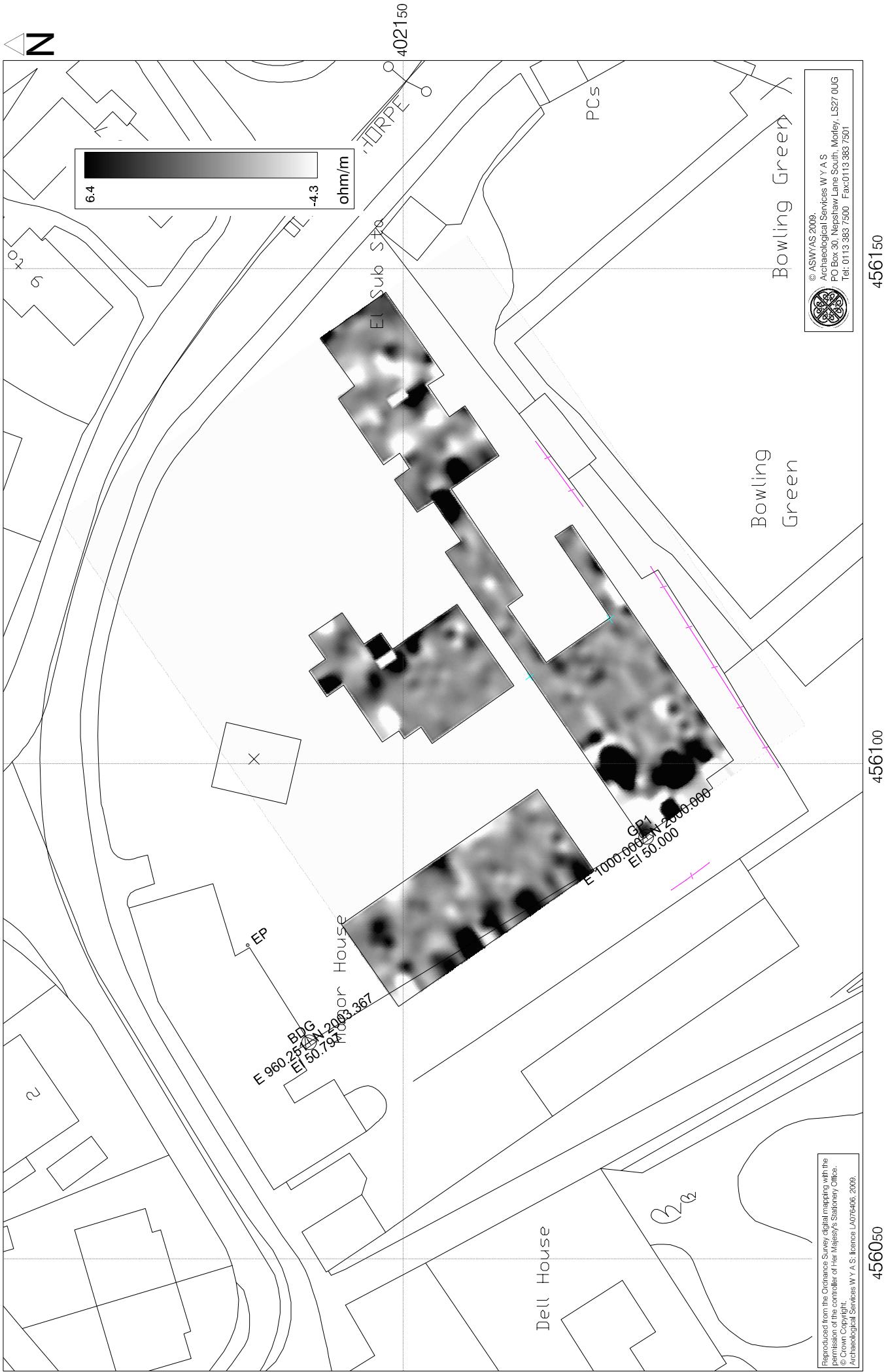
Fig. 6. Processed greyscale earth resistance data (1:500 @ A4)
