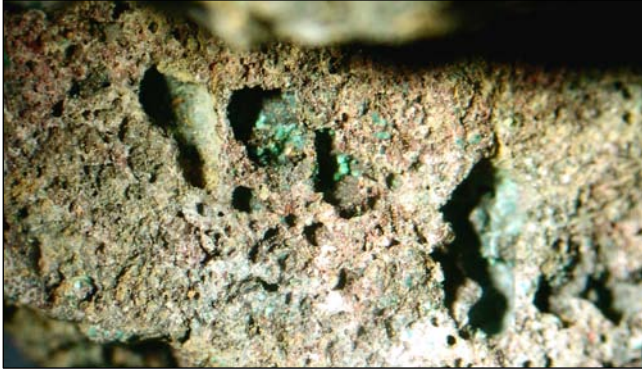
Plate 15. Chemically bonded corroded copper alloy within the fabric of crucible 3 (1271) (x16) (Photo: J. Jones)
