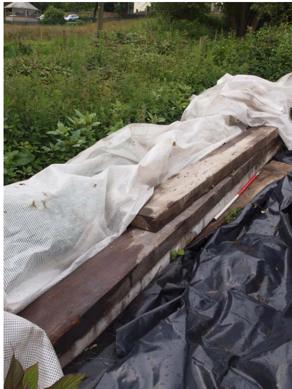
Plate 25: Machine cut timber purlins
