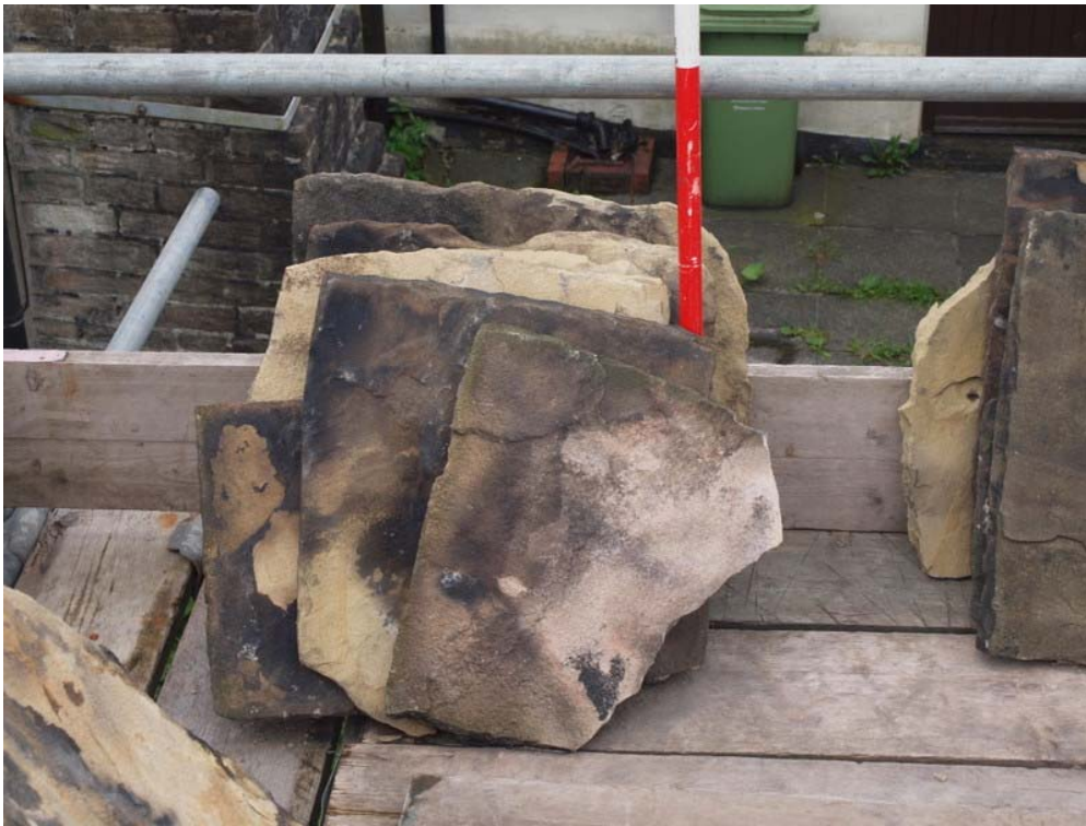
Plate 41: Sandstone roof slabs
