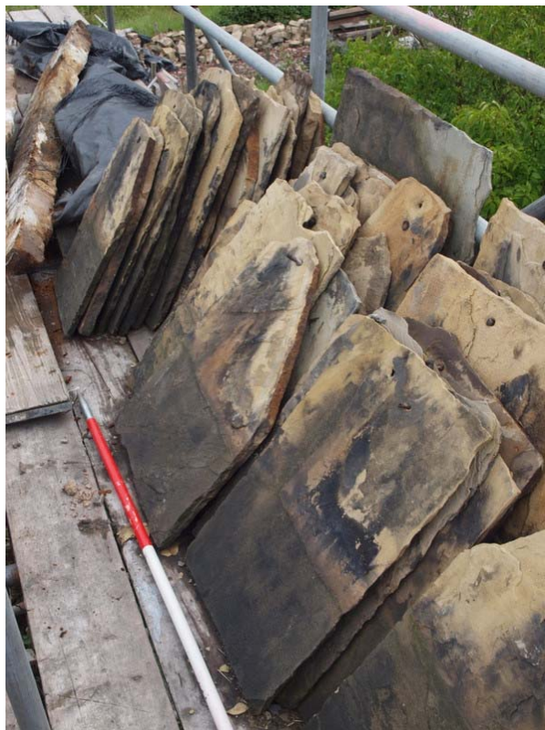
Plate 44: Sandstone roof slabs
