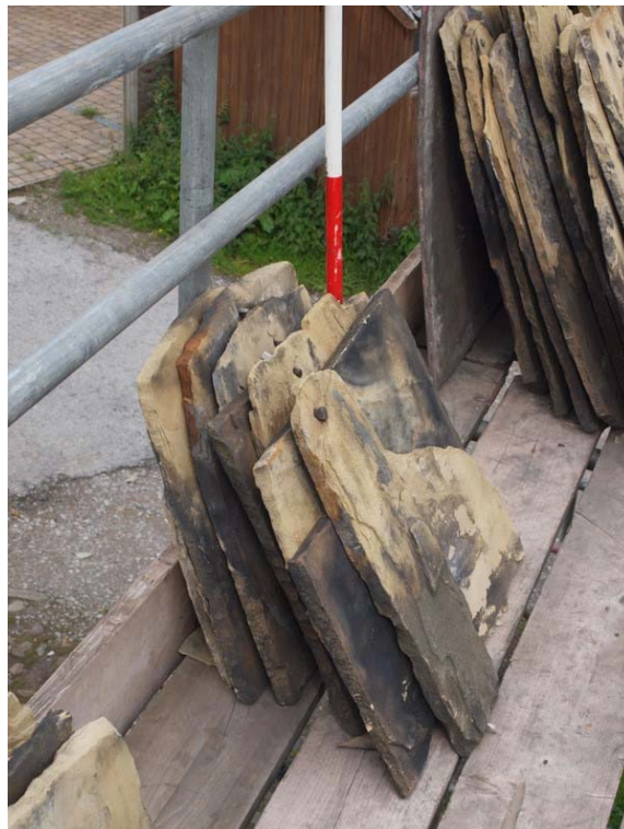
Plate 38: Sandstone roof slabs
