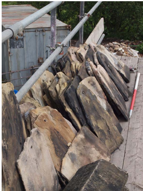
Plate 34: Sandstone roof slabs
