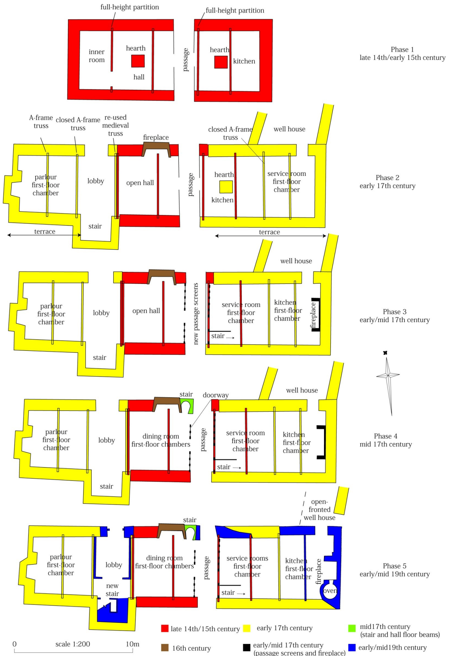
Fig. 1 Phase plans showing suggested development of the house up to the mid 19th century, including roof trusses.
