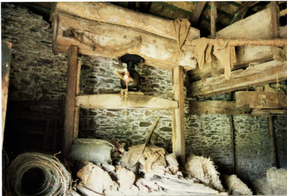
Plate 30. Cider press and milling machinery in barn.
