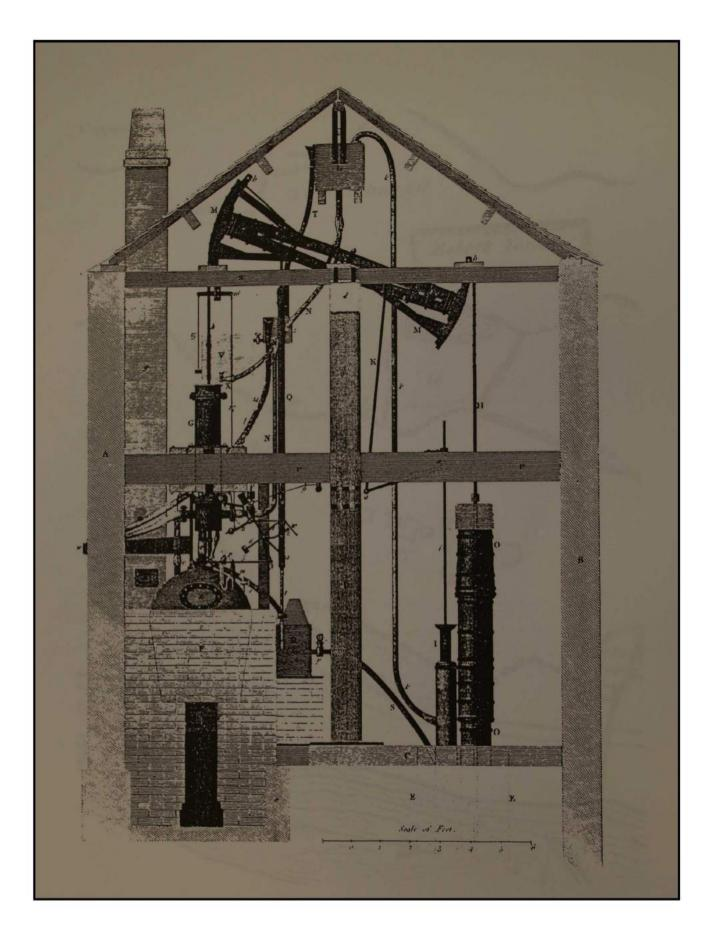
Fig 4.13: An early Newcomen pumping engine showing the boiler directly beneath the cylinder after Rees 1819-20, quoted in Heyman 1996
