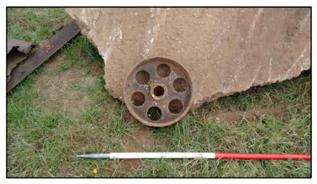
Fig 40: Pully wheel for shaft drive
