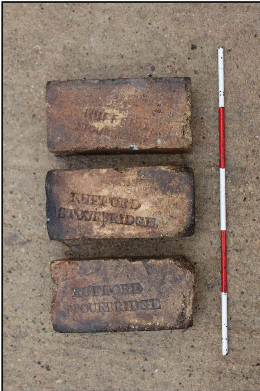
Fig 24: Samples of bricks from the site; made by Rufford of Stourbridge, scale 0.5m
