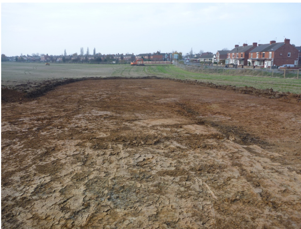
Plate 2. Variations in the natural in the south-eastern area strip, with clay in the foreground and fractured sandstone beyond.
