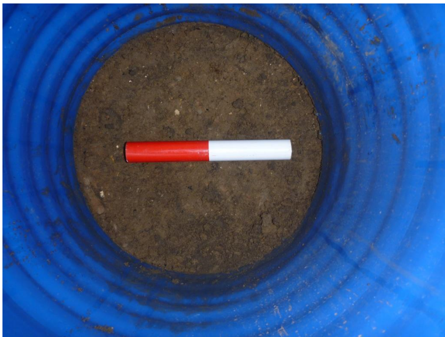
Plate 7 Motte make-up material exposed at base of geotechnical inspection pit
