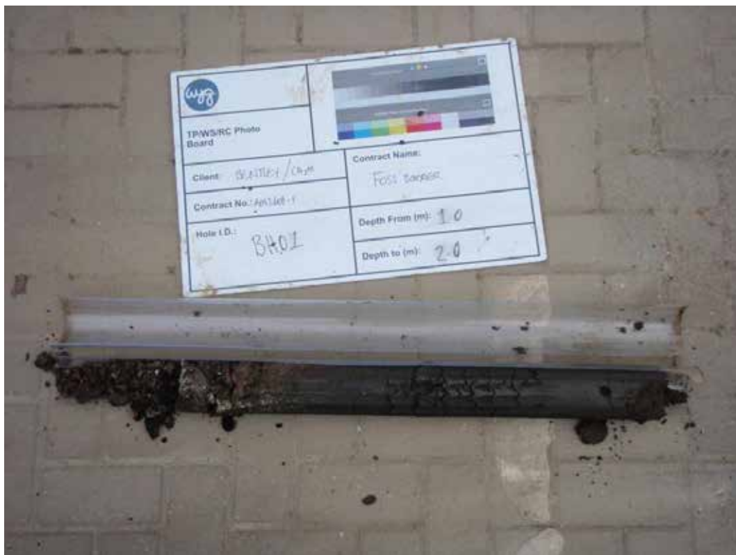
Plate 5: Borehole 1 (Window sample sleeve 1-2m, 2m depth to the right)
