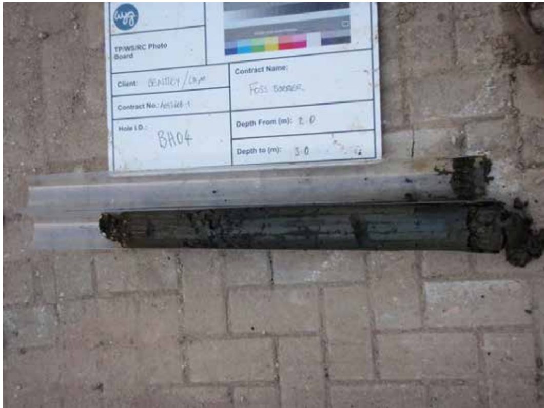
Plate 3: Borehole 4 (Window sample sleeve 2-3m, 3m depth to the right)
