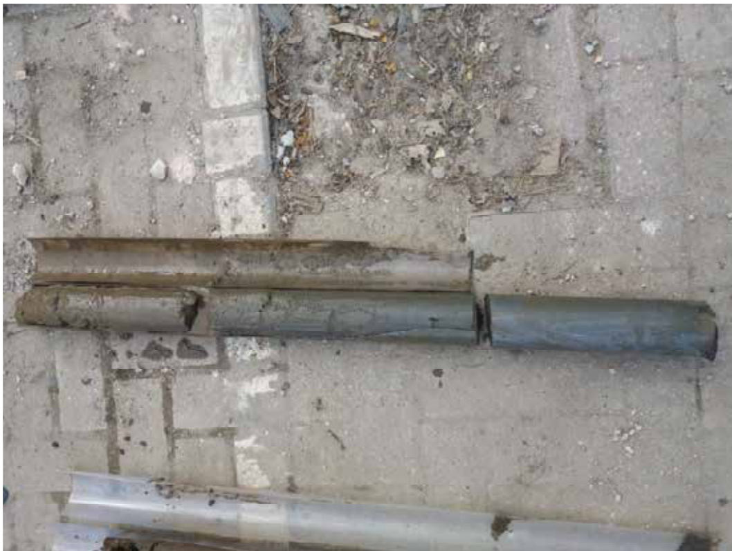
Plate 4: Borehole 6 (Window sample sleeve 4-5m, 5m depth to the right)
