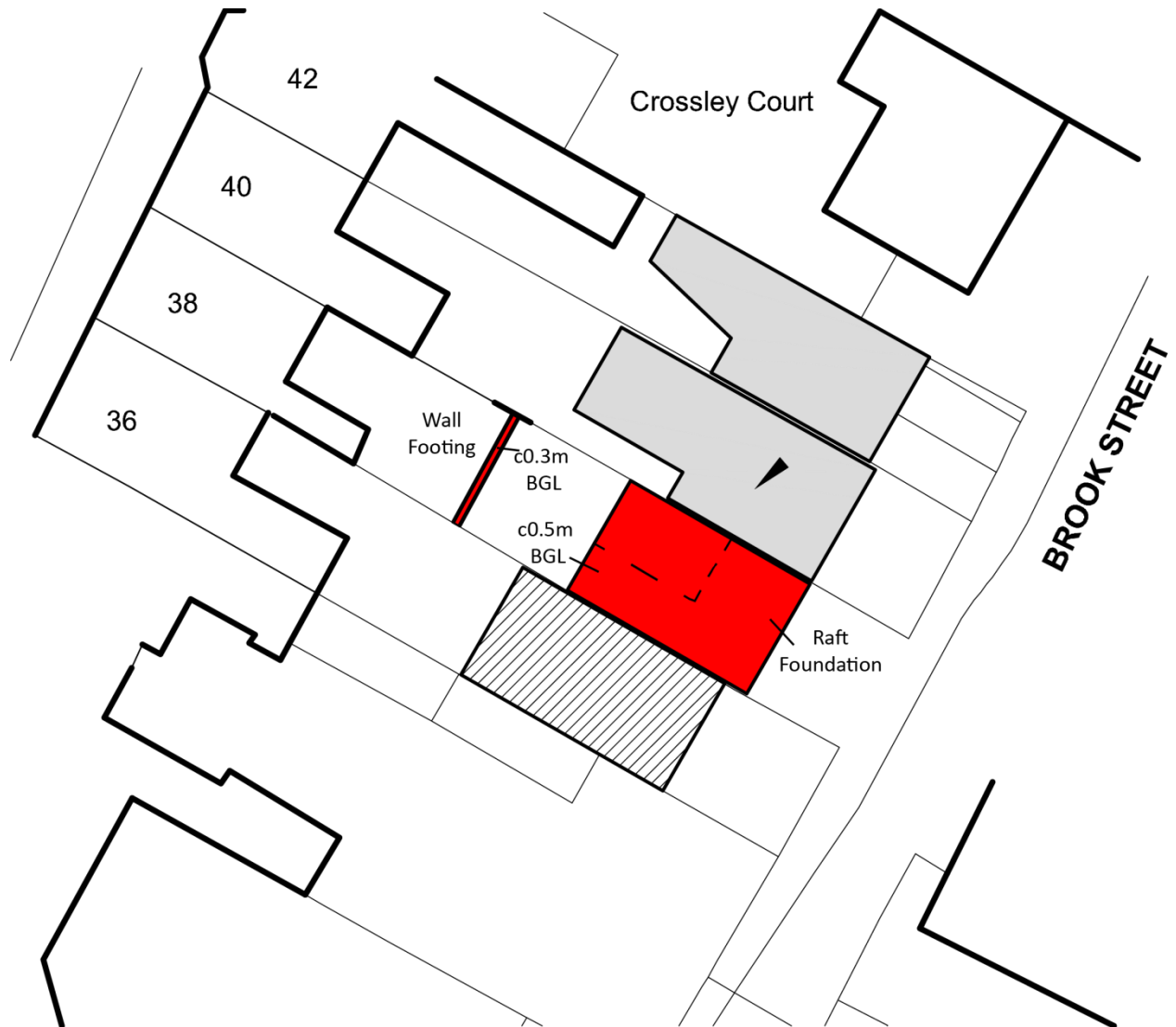
Figure 2: Layout of excavations at 1:250 Scale (Area enclosed by dashed line not observed)
