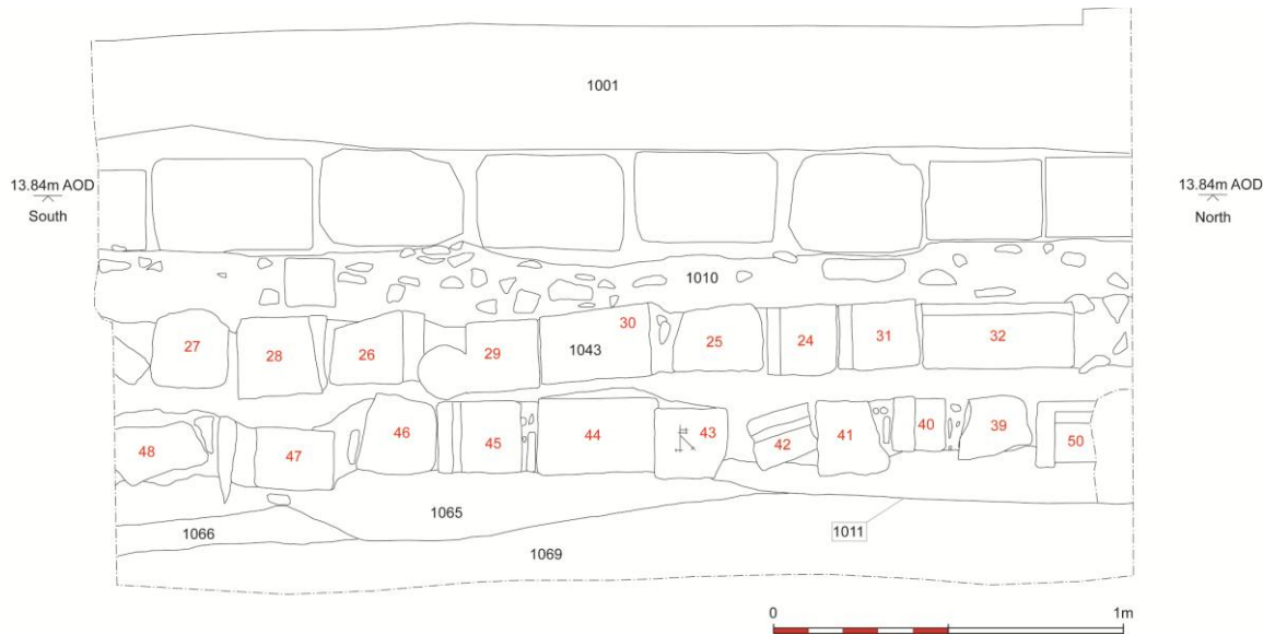
Figure 11 East facing elevation of west wall foundation, prior to stone removal, with removed stones numbered in red
