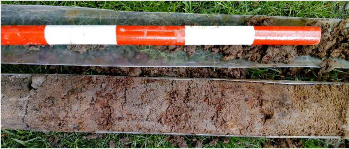
Plate 19 WS02 core 1m–2m, top to the left, showing (l–r) contexts 202–204. Iron pan can be seen on context 202 and 203. Scale 0.5m
