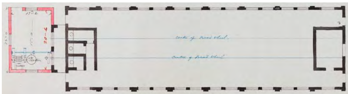
Plate 23 Detailed plan of the treadmill including the addition of the grain mill to the south. From proposed plans from 1870.
