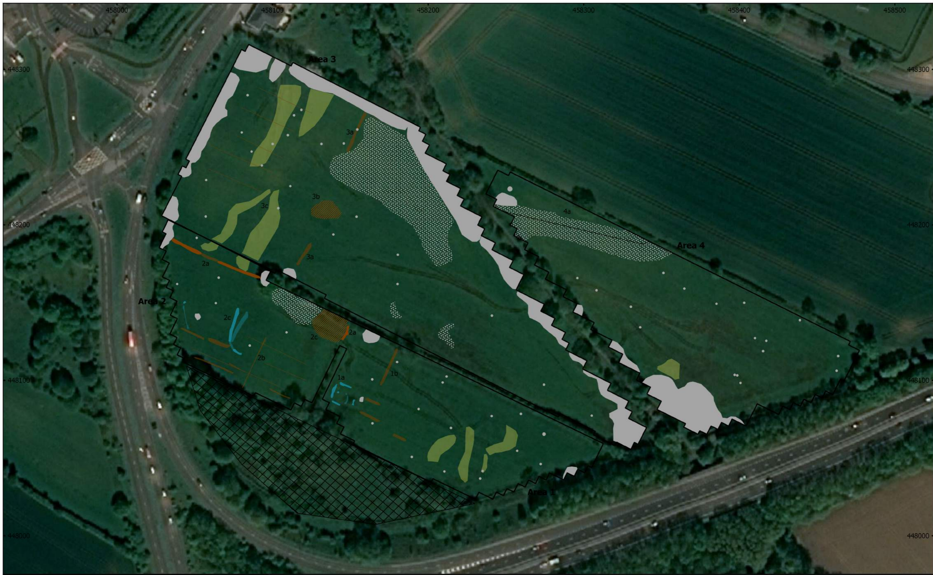
MSSE335 - Tadcaster Road, Ashfield Estate Land Figure 6 - Magnetic Interpretation Over Satellite Imagery 1:1500 @ A3 Copyright Magnitude Surveys Ltd 2018 Contains satellite imagery © 2018 Bing Satellite
