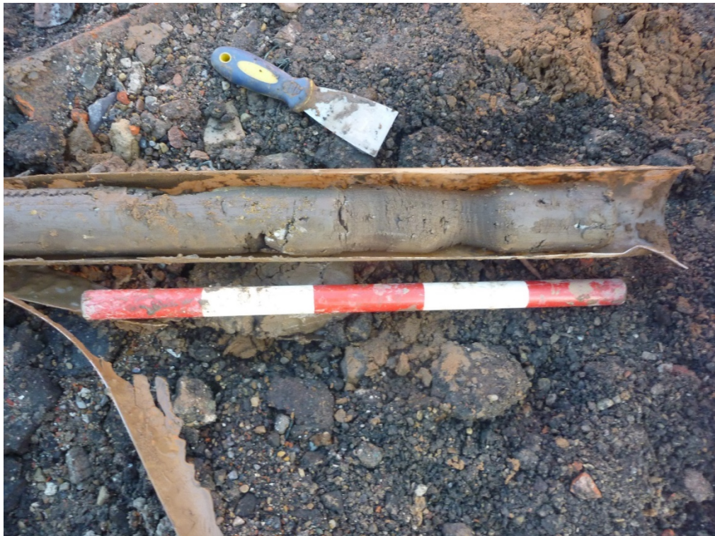
Plate 6 Sample from between 4m and 5m BGL in BH03. Natural boulder clay.
