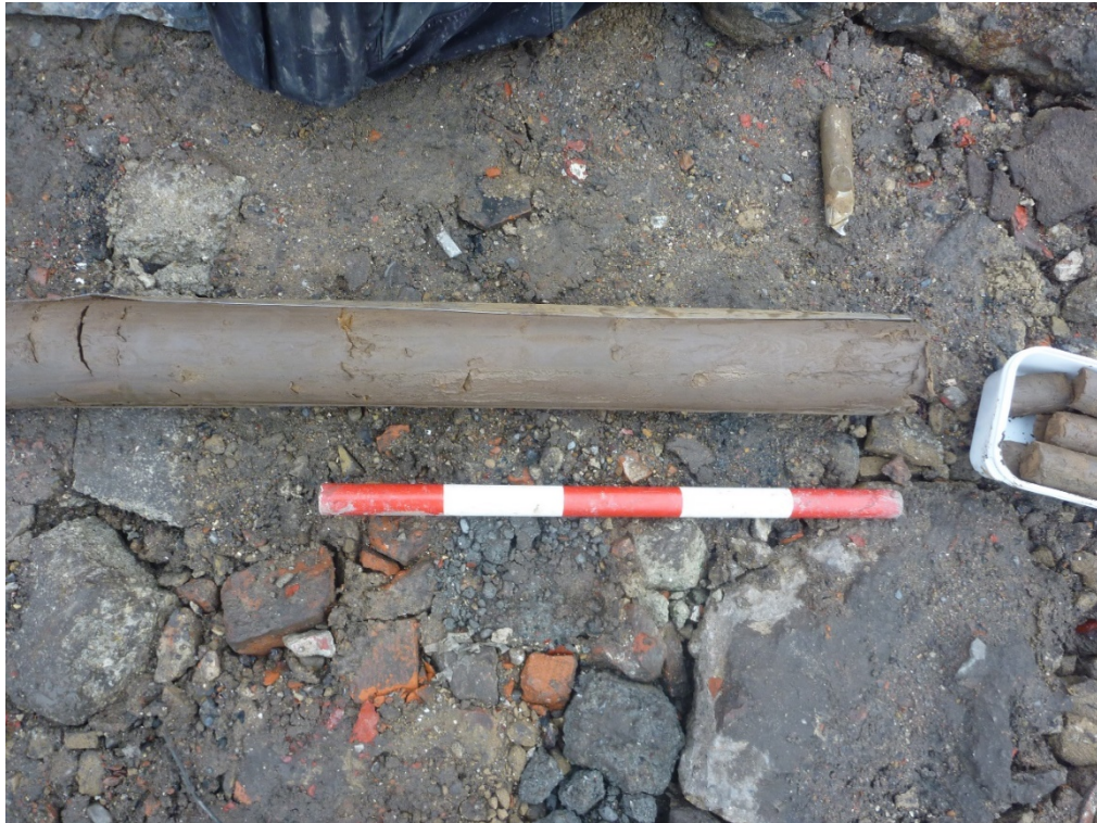
Plate 5 Clay/sand laminates between 0.7m and 2.6m BGL in BH02.
