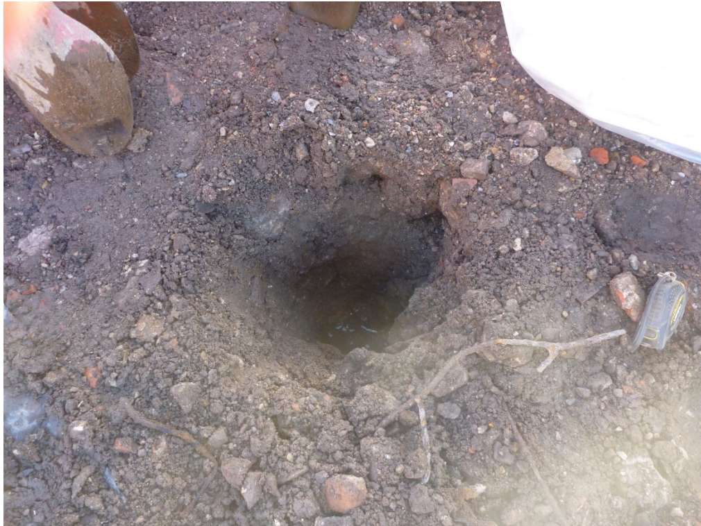
Plate 9 Hand dug test pit of first metre in BH04. Standing water where obstruction was encountered resulting in the borehole being abandoned.
