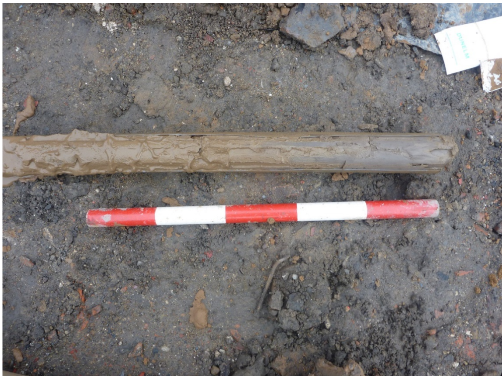
Plate 2 Boundary between the clayey sand made ground (C203) and natural Boulder Clay (C204). Encountered at 4.7m BGL in BH02.
