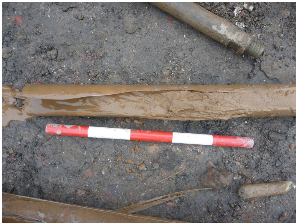
Plate 3 Clayey sand made ground deposit in BH02 (C203), same as visible in BH01, Plate 1.
