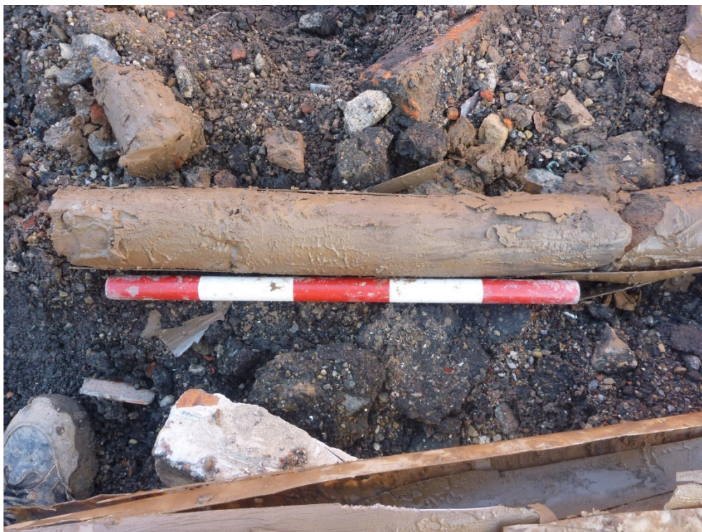
Plate 7 Boundary between clayey sand made ground and natural boulder clay in BH03. Natural was encountered at a much shallower depth of 3.5M BGL compared to the boundary in BH02 (Plate 2).
