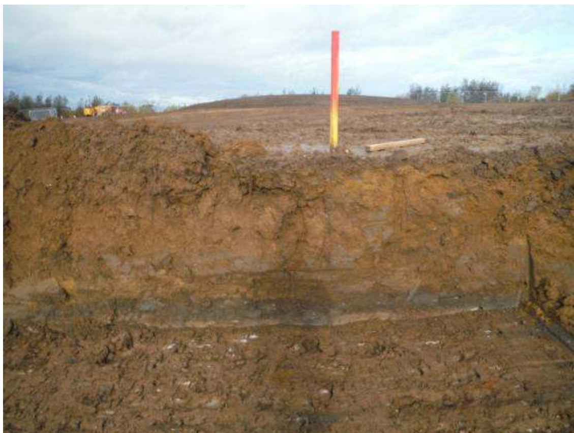
Plate 4. Typical cross-section view showing landscaping dump overlying disturbed topsoil and natural clays. Facing north-west.
