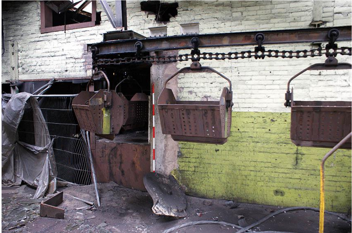
Plate 27: Bucket line, part of No. 7 mould line, going into main area of building 7
