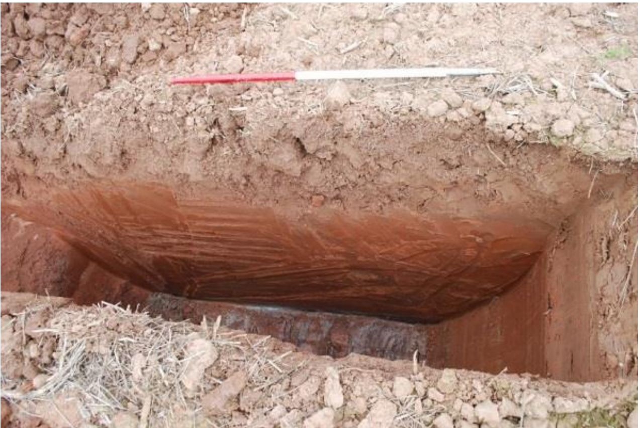
Plate 15 Example of topsoil, marl and solid Mercian mudstone sandstone in geotechnical pit
