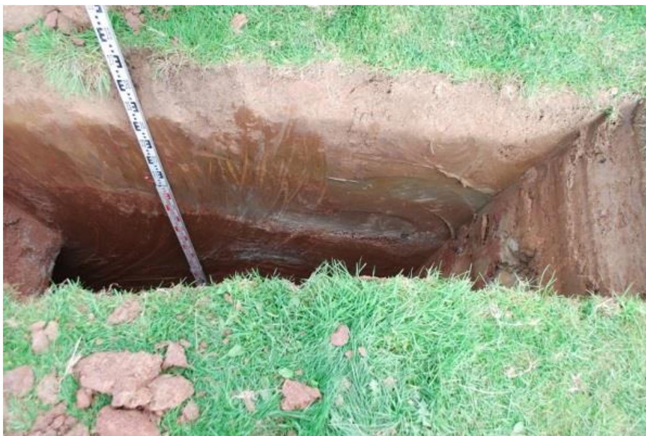
Plate 16 Grey clay in TP207 overlain by clay and topsoil.
