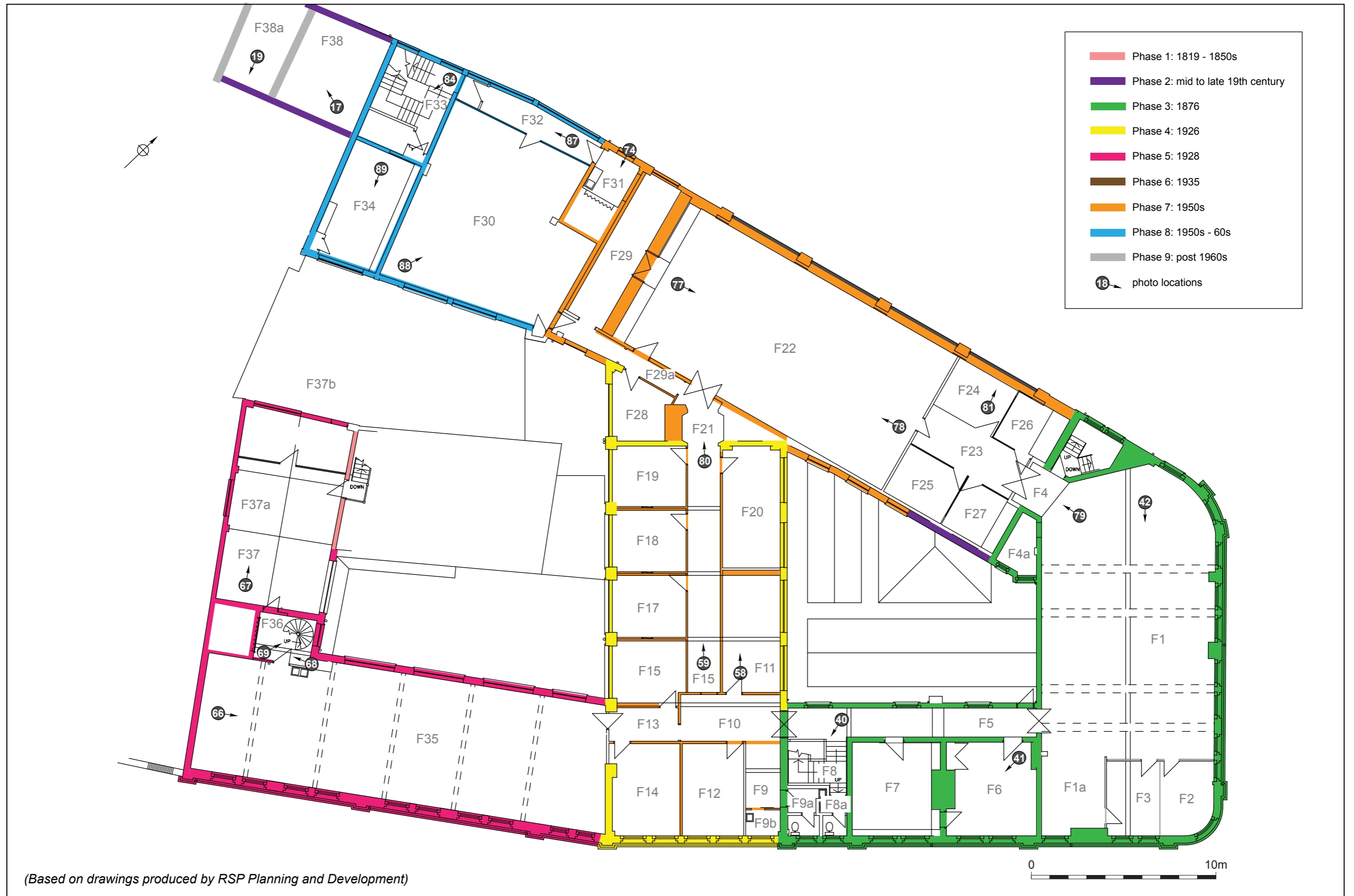
First floor plan of Brinton's Office (with room numbers) showing phases and photo locations
