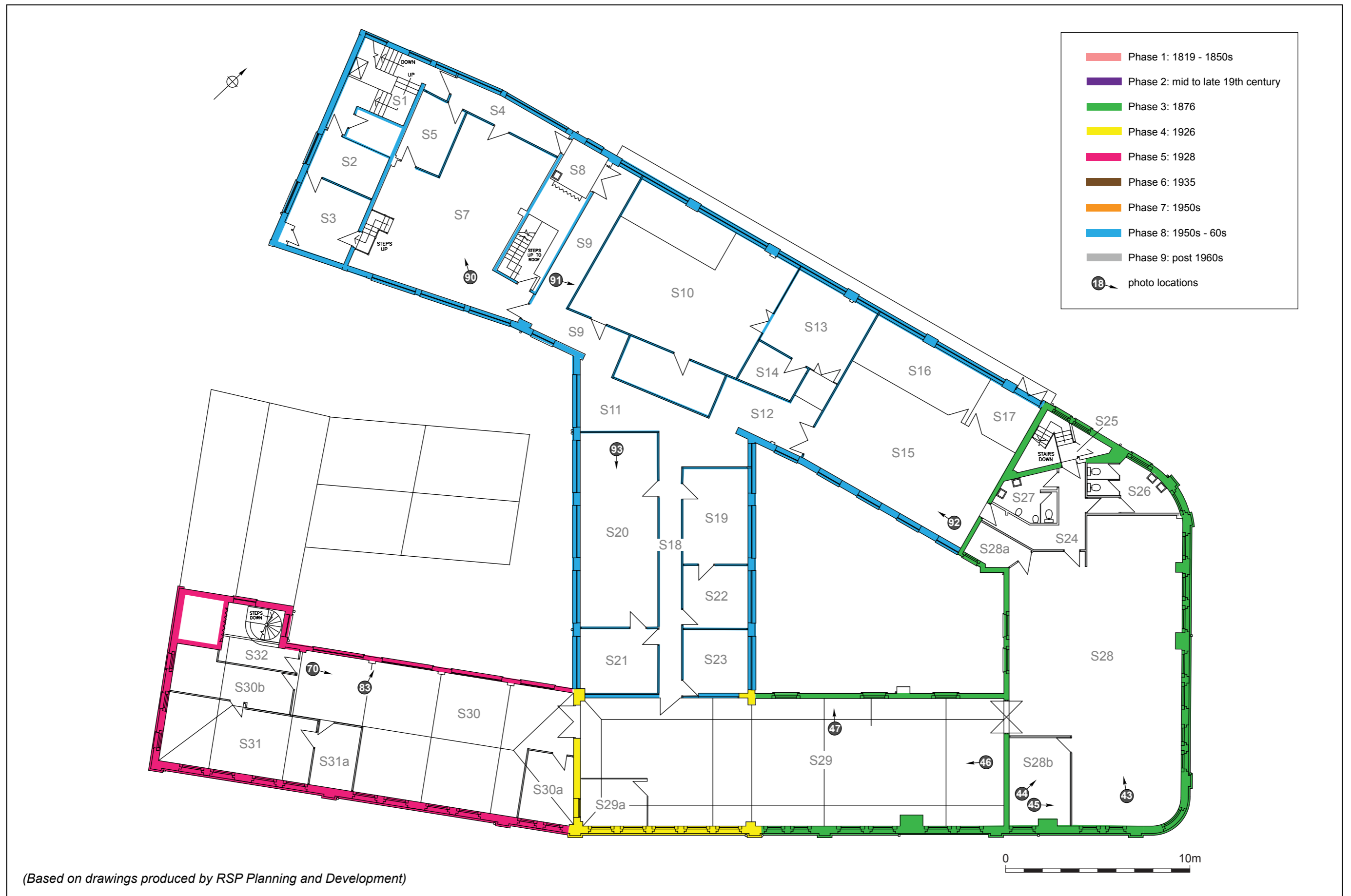
Second floor plan of Brinton's Office (with room numbers) showing phases and photo locations
