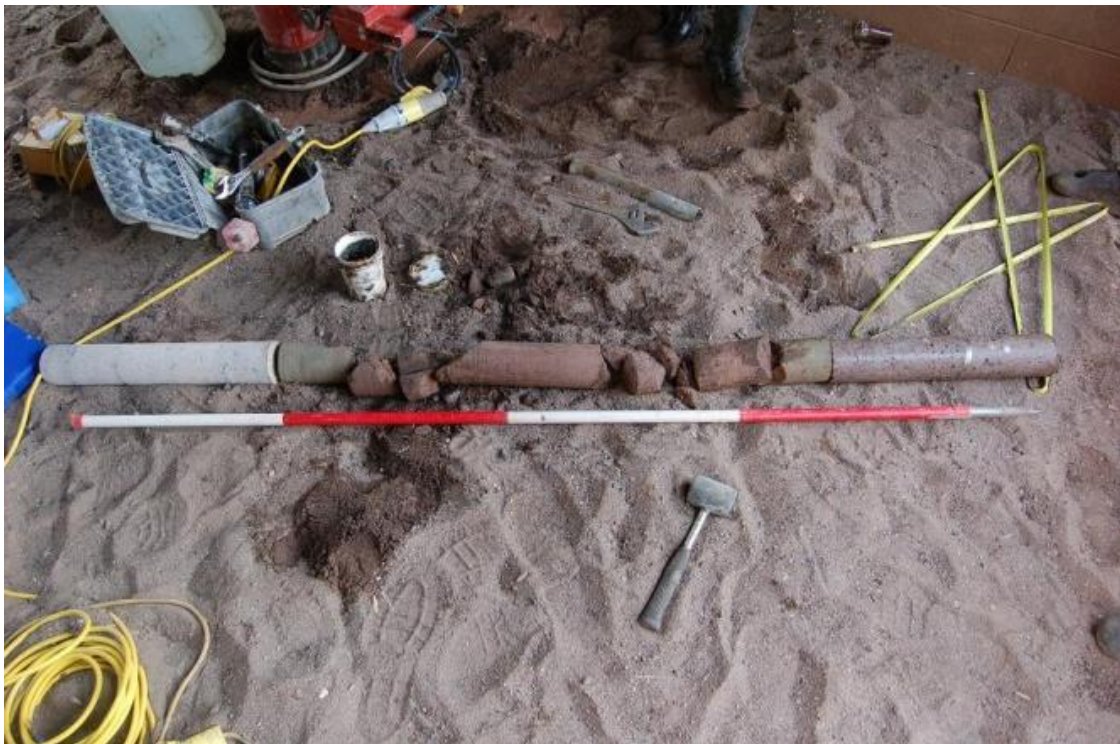
Plate 22 Parts of the core through southern pier (2.56m in total) showing reinforced concrete at either end, and green sandstone encasing red sandstone at the centre
