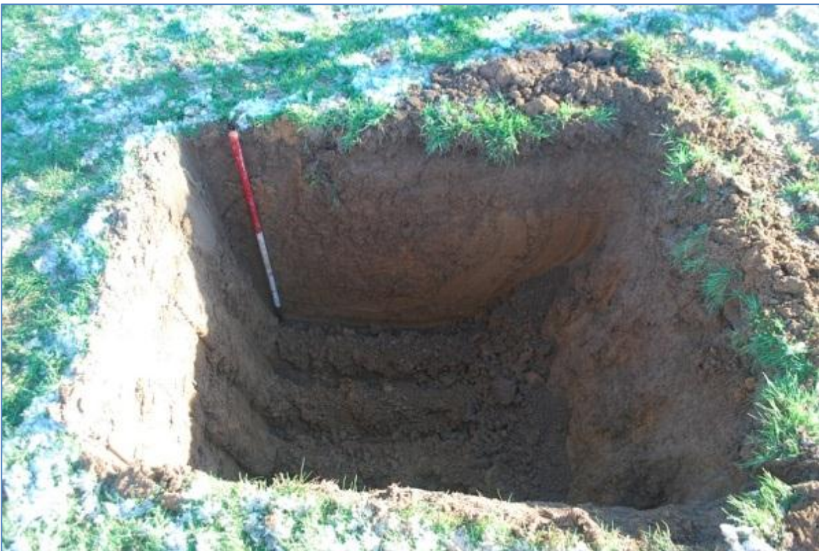
Plate 2 An example of a geotechnical test pit in the south east corner of the site
