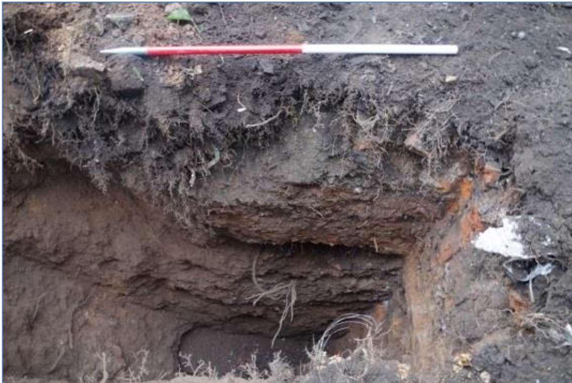
Plate 6 Geotechnical pit 14 showing made ground
