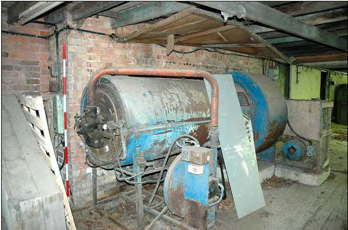
Plate 17: Early 20 th century kiln with segmental head opening into furnace area
