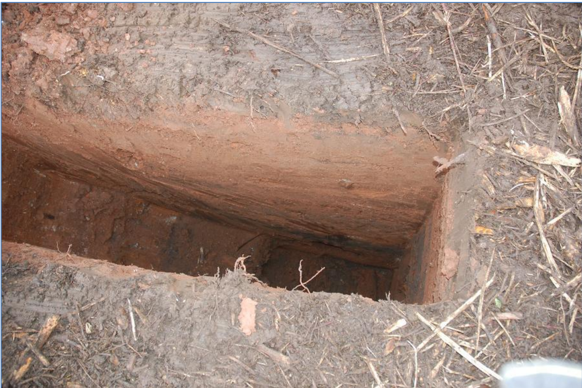
Plate 2 Trial hole 2 4.1m total depth demonstrating redeposited Mercian mudstone, clays and 20 th Century rubble material, view of south facing section
