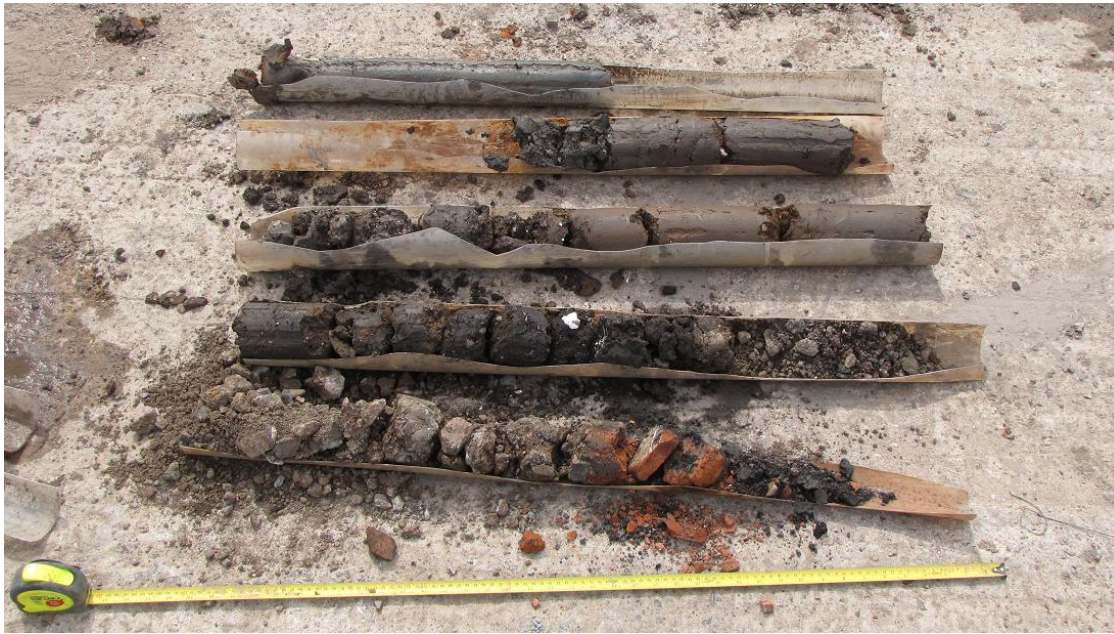
Plate 1 Borehole 5 geotechnical sequence (opened on site for contamination analysis)
