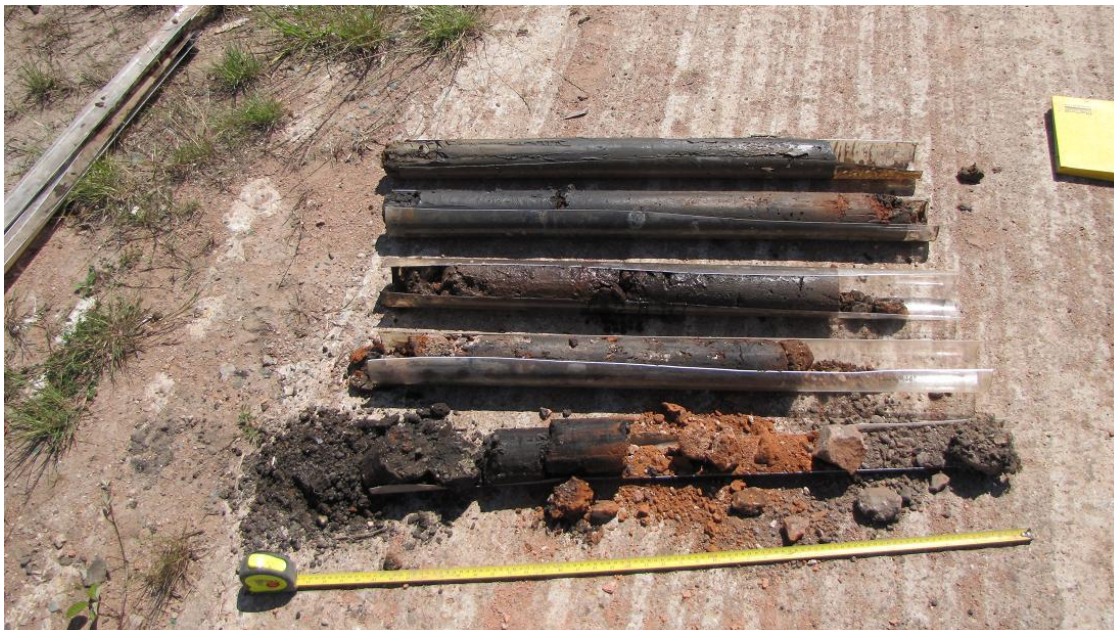
Plate 2 Borehole 6 geotechnical sequence (opened on site for contamination analysis)
