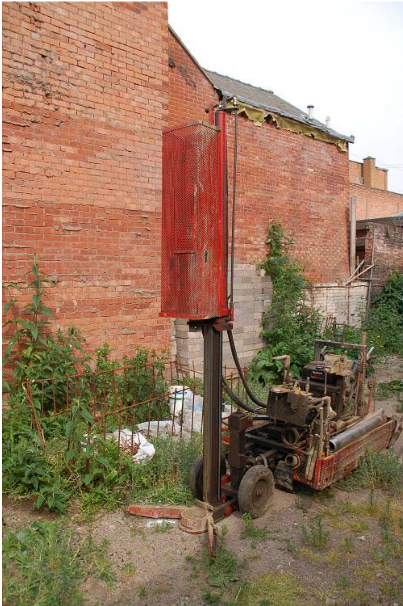
Plate 3 The percussive rig in use
