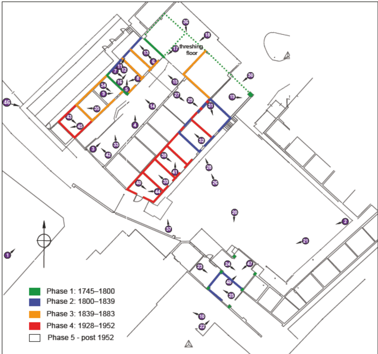
Phase plan with photo locations based on Nick Carroll Architects drawing number 1517/02-03
