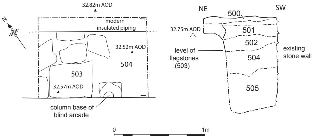
Plan and section of Test Pit A; Section of Test Pit B.
