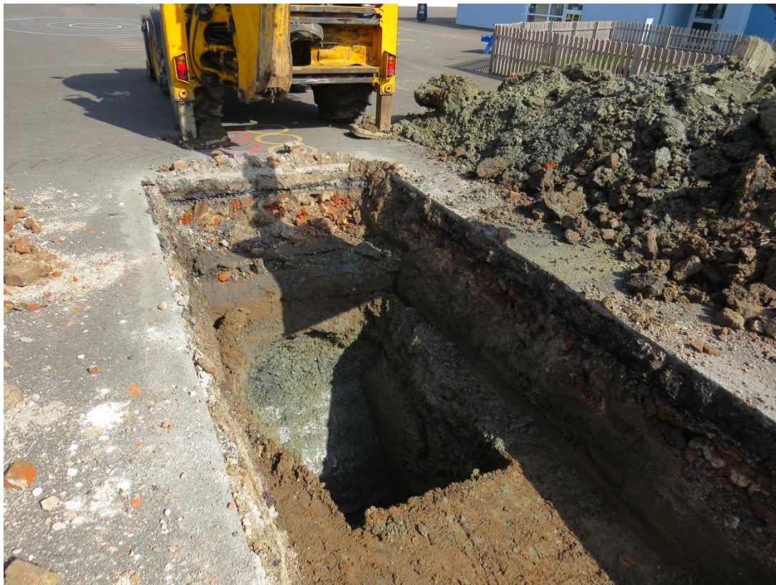
Plate 4. North face of TP 4 showing made ground underlain by tri-partite sequence of Holocene alluvium, sand and gravel, and alluvium.
