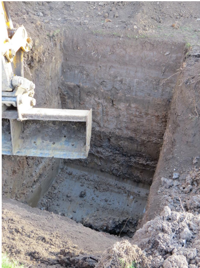
Plate 5. South face of TP 5 showing tri-partite sequence of Holocene alluvium, sand and gravel, and alluvium.
