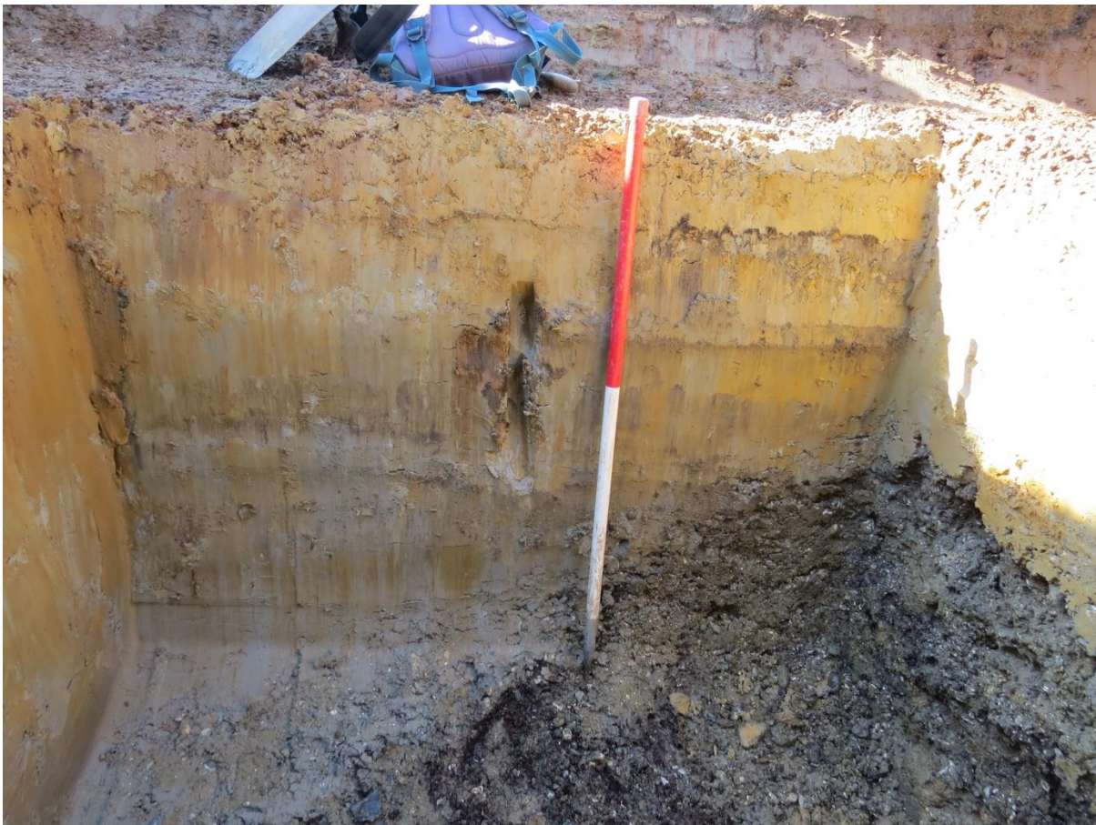
Plate 7. West face of TP 7 showing stratigraphy of alluvium onto Pleistocene sands and gravels.
