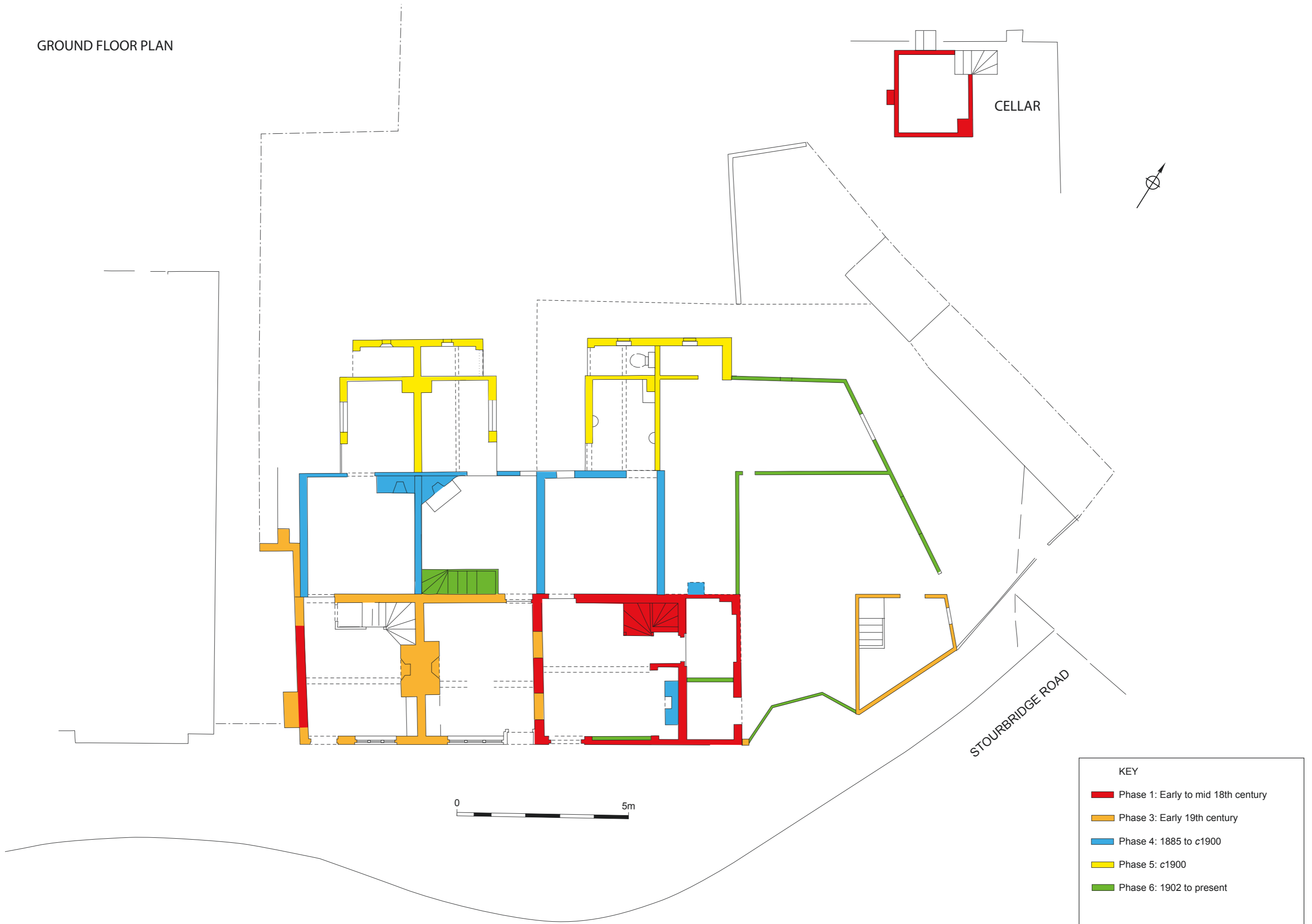
Ground floor plan with phasing (based upon Rodney Melville + Partners Drg No 11)
