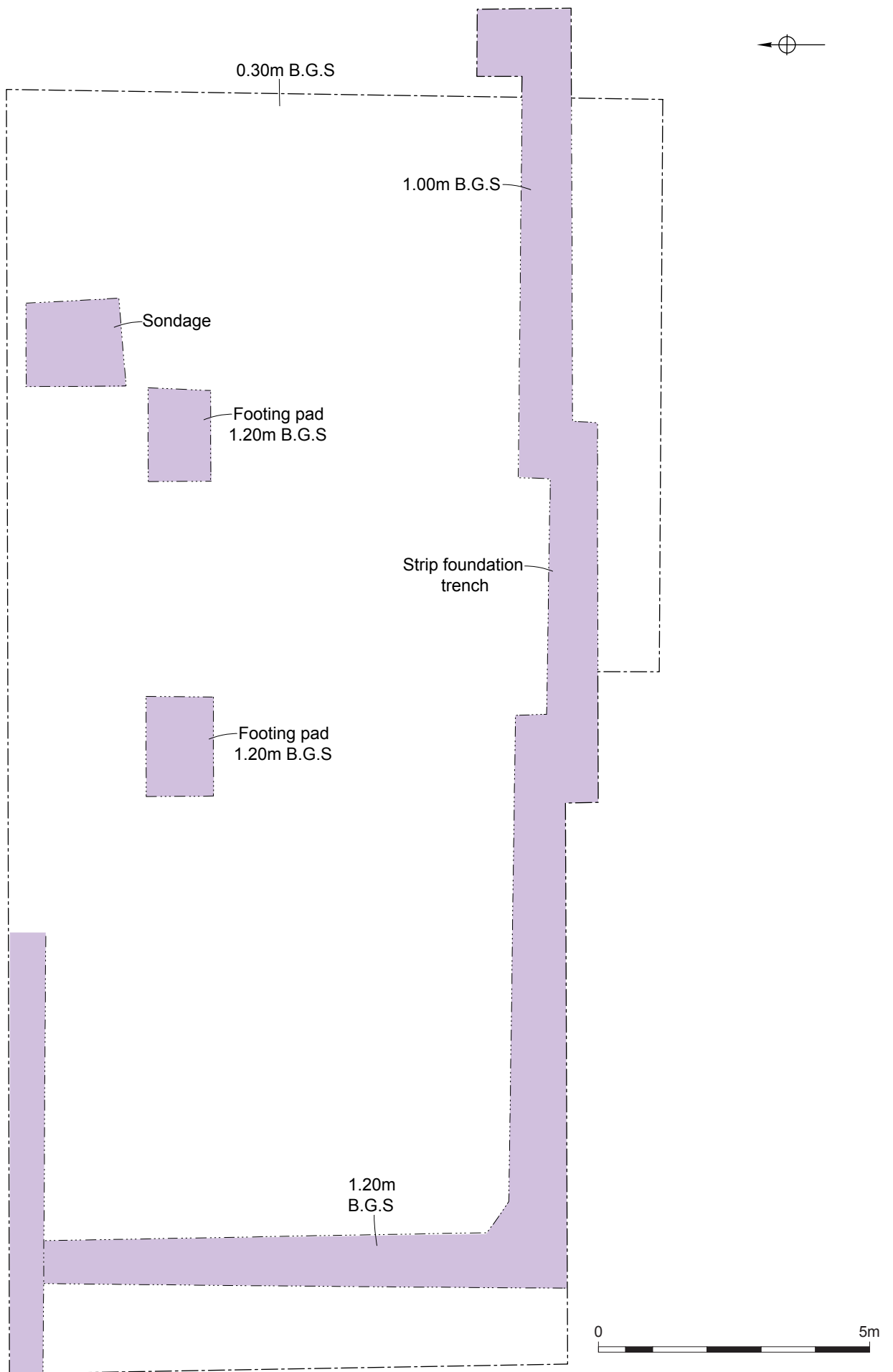
Trench 1: groundworks for new building
