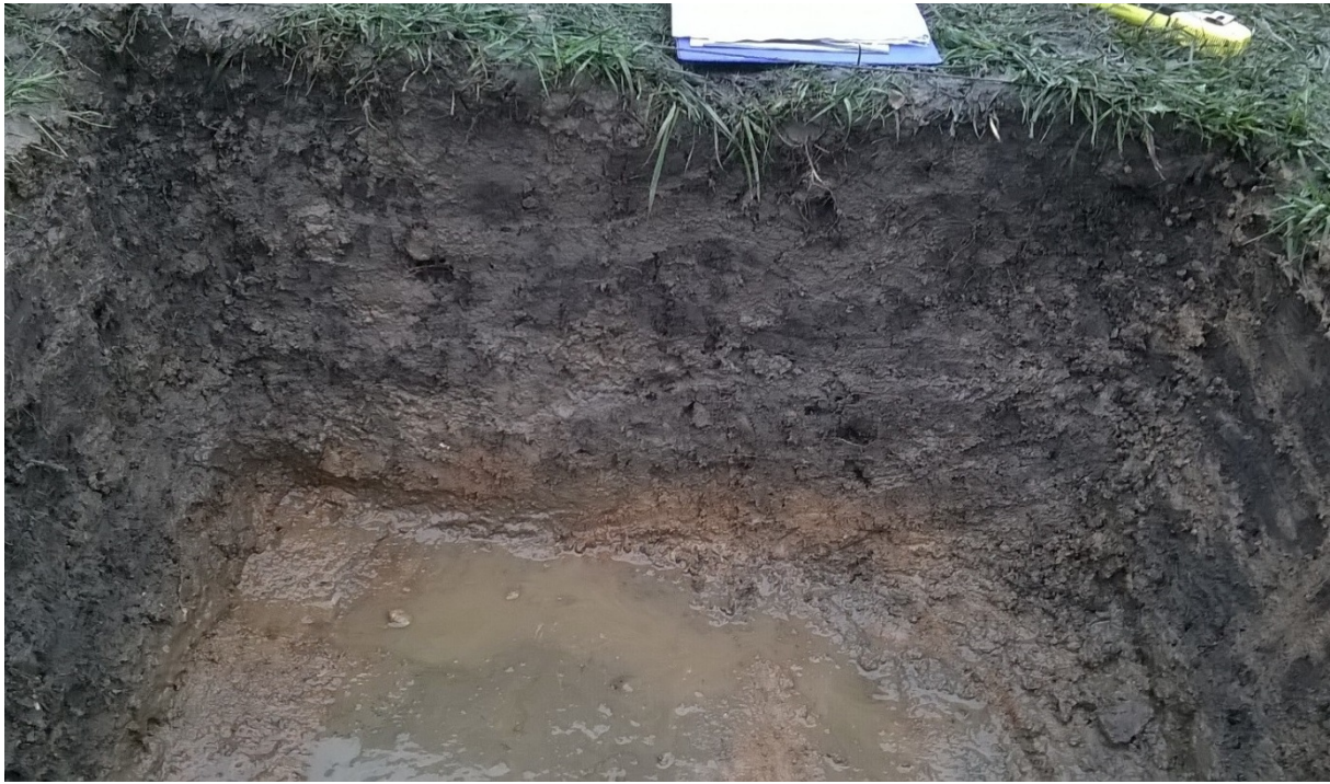
Plate 7: Side of Test Pit 7 showing thick dark layer of household rubbish and lighter layer below just beginning to appear – photo looking east
