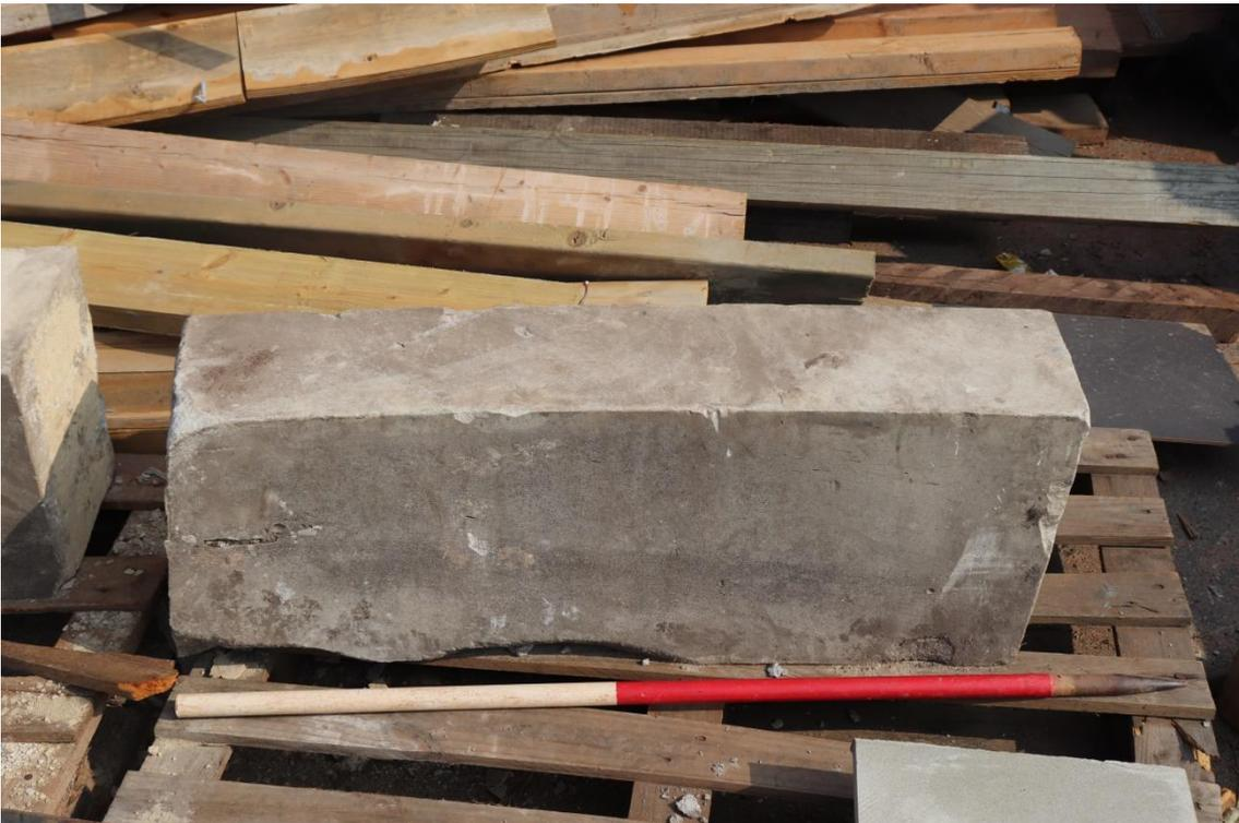
*Plate 19 Pillar stone with evidence of circular saw conversion*
