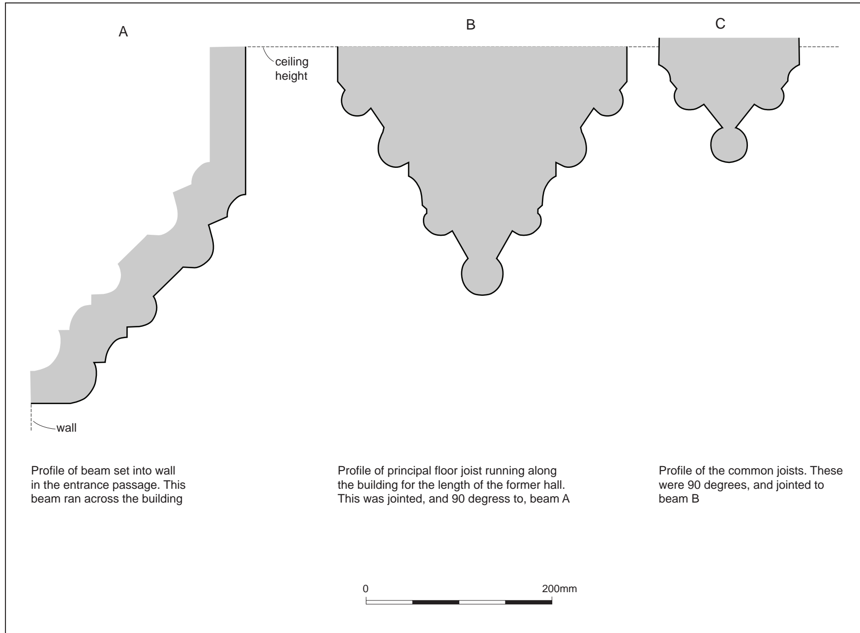
Phase 1 ceiling beam mouldings above the former hall
