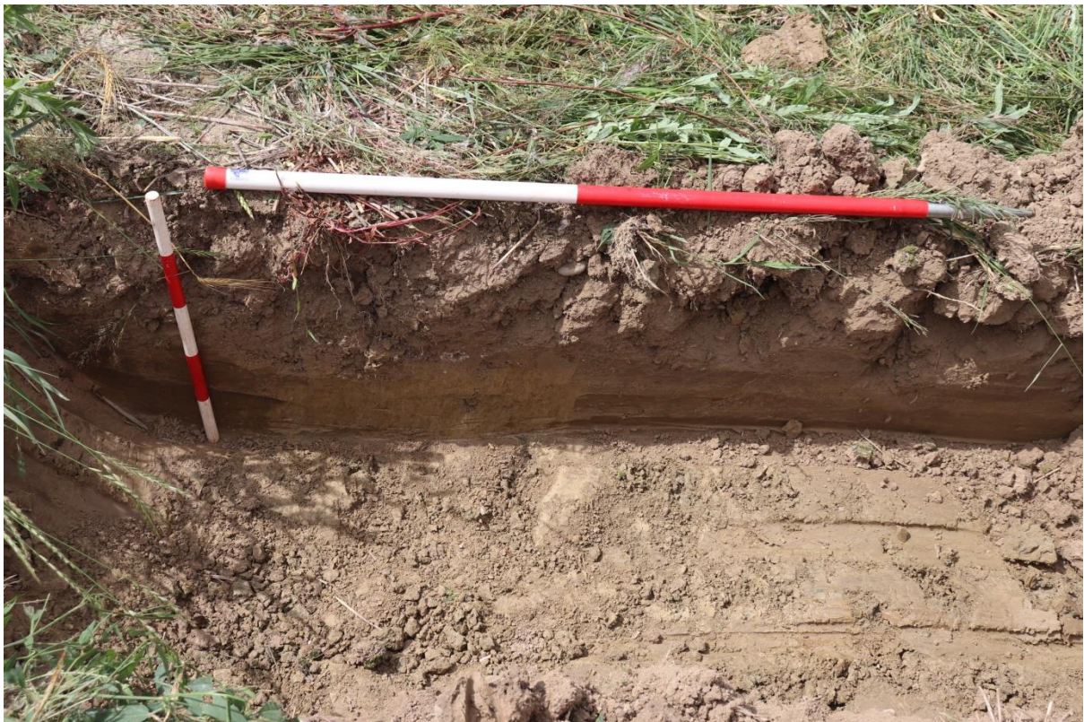
Plate 8: Soil profile for bat barn Trial hole TP101. 1m and 0.5m scales.
