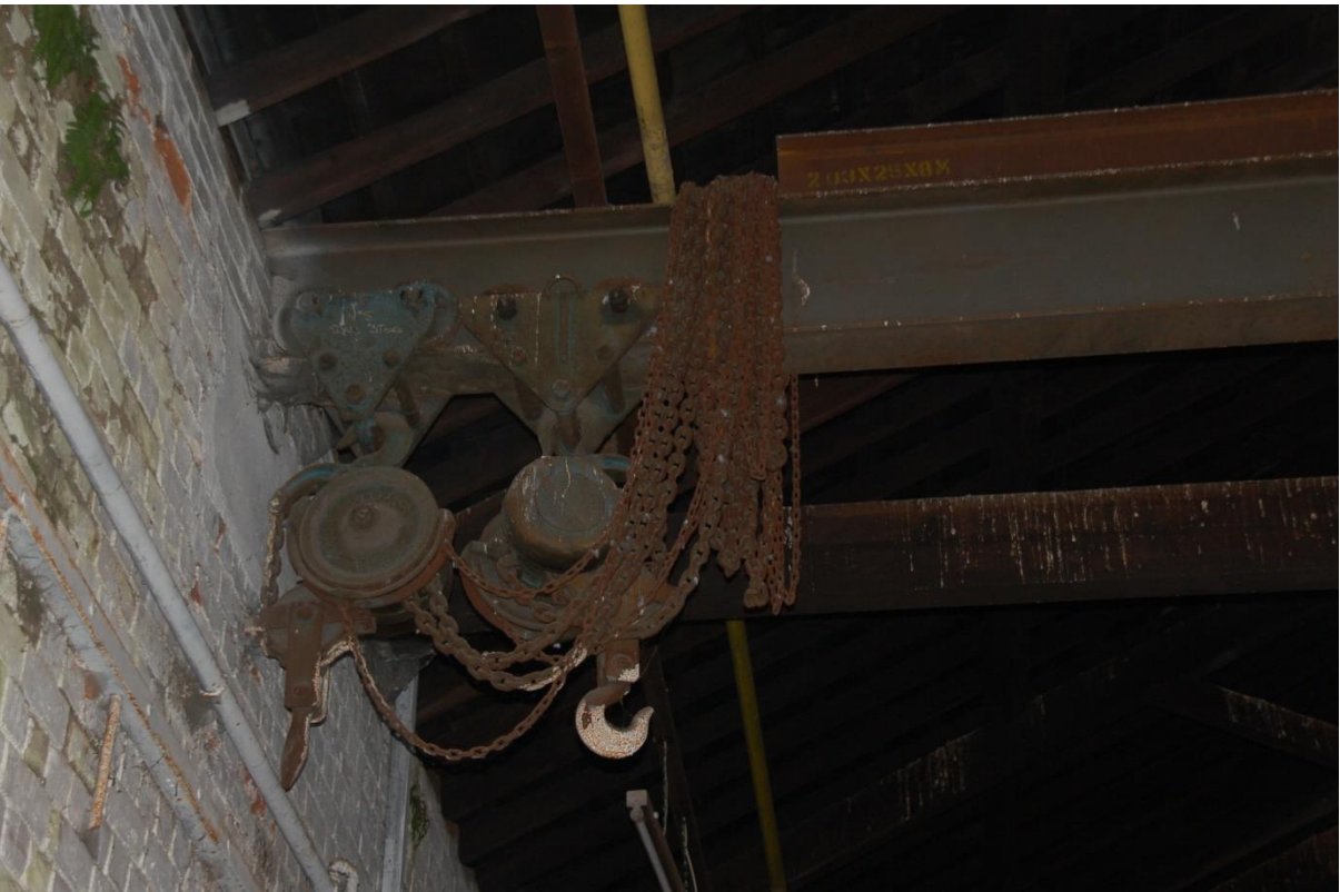
Plate 23 Half-ton Yale Model BB Spur Geared Block Manual Chain Hoists in Acidifying shed B2
