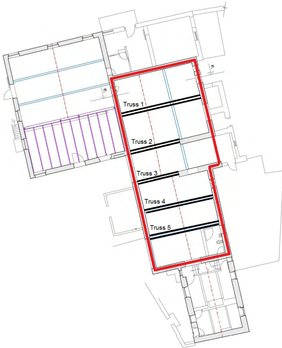
Figure 3: Plan showing the of range of buildings with the barn outlined in red and the trusses marked and numbered (Bennett-Ing's Developments Limited)
