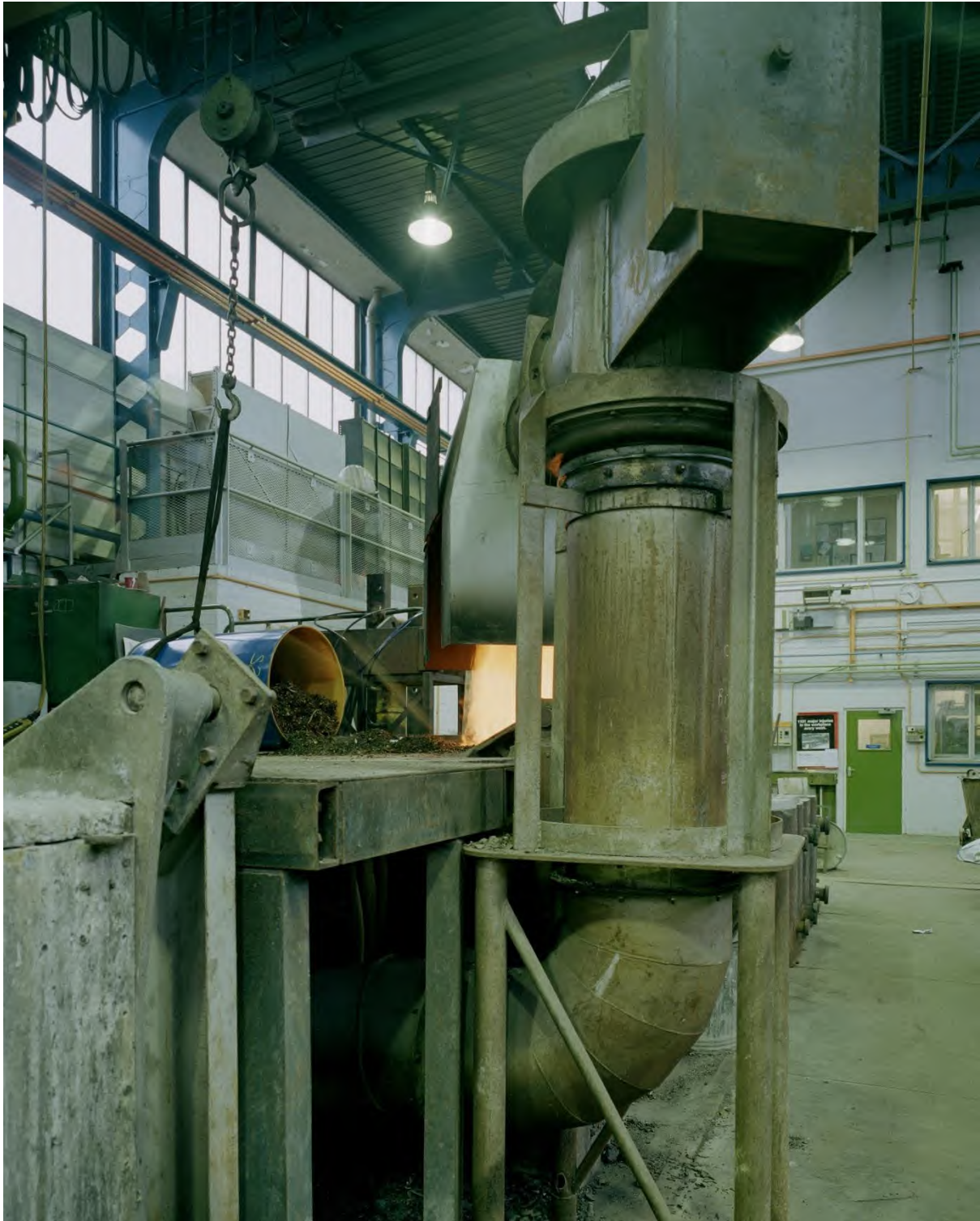
AA040578 F Block - small high frequency furnace used to assay scrap metal (copyright Historic England Archive 2002)
