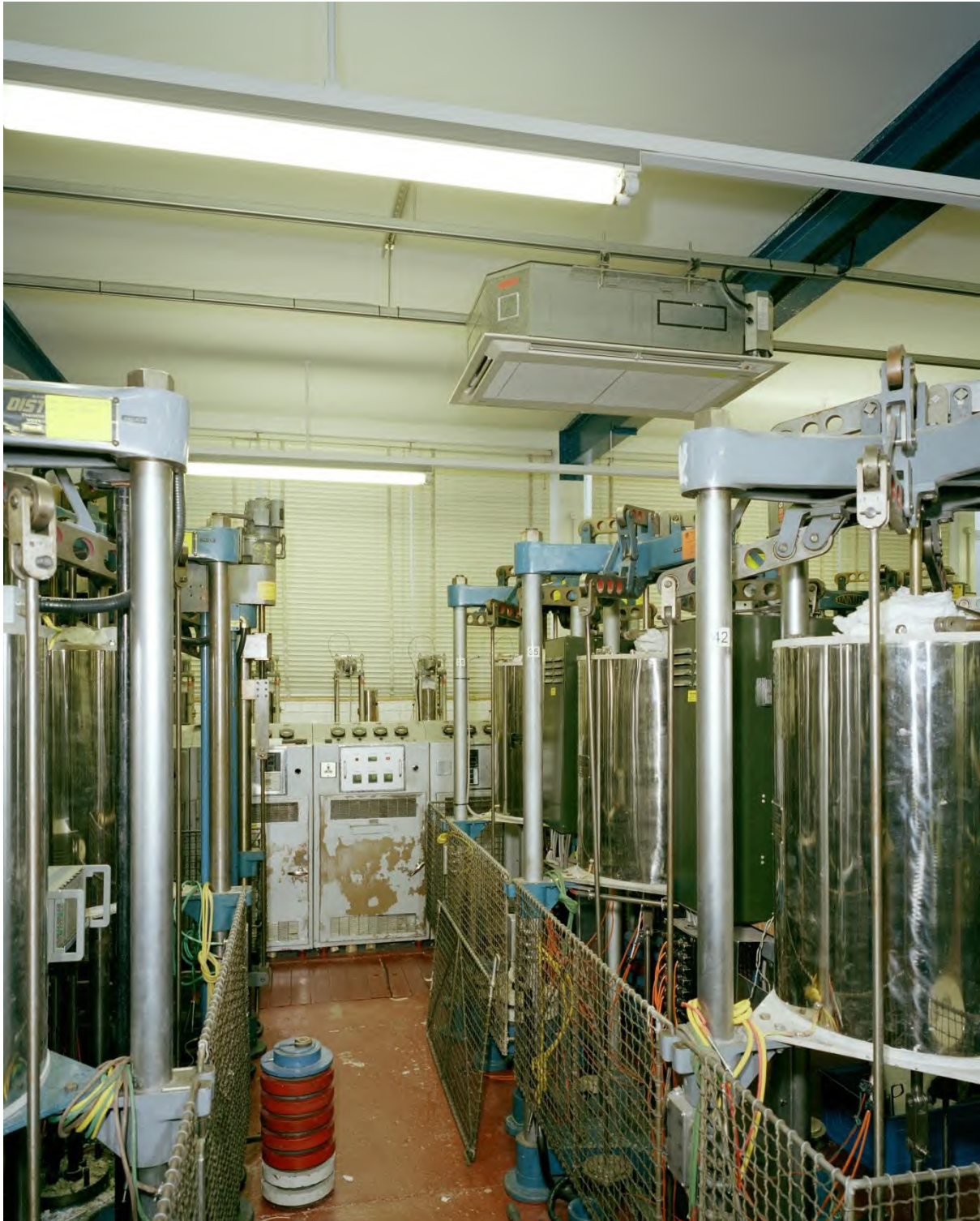
AA040594 Block A – creep testing laboratory, studying the deformation of metal over a long time including some continuing experiments commenced in 1958 (copyright Historic England Archive 2002)
