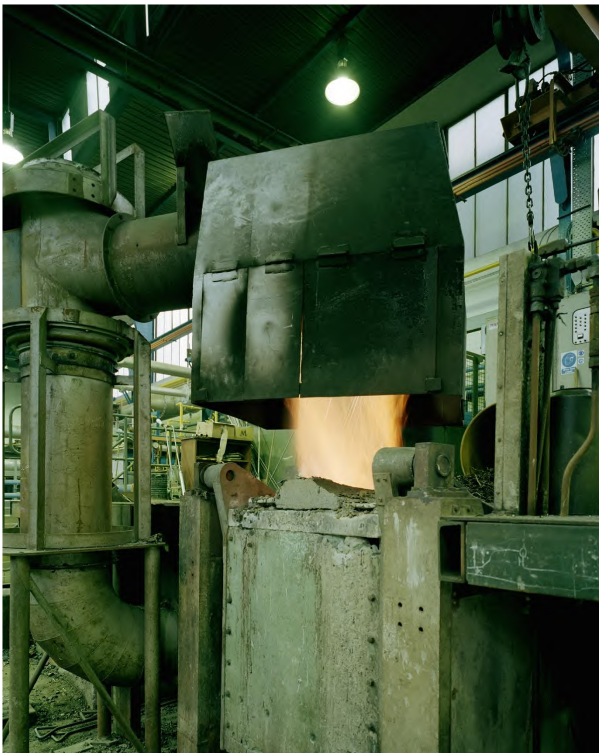
AA040579 F Block - melting scrap metal prior to forming ingots for testing (copyright Historic England Archive 2002)
