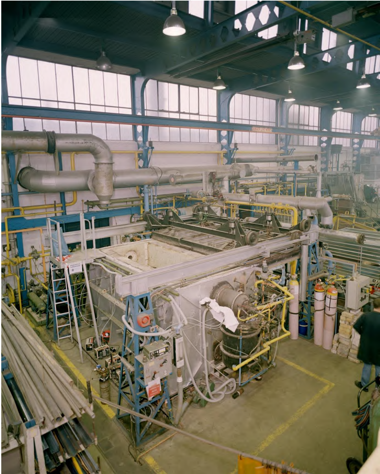
AA040584 F Block - soaking pit for reheating ingots prior to rolling (copyright Historic England Archive 2002)
