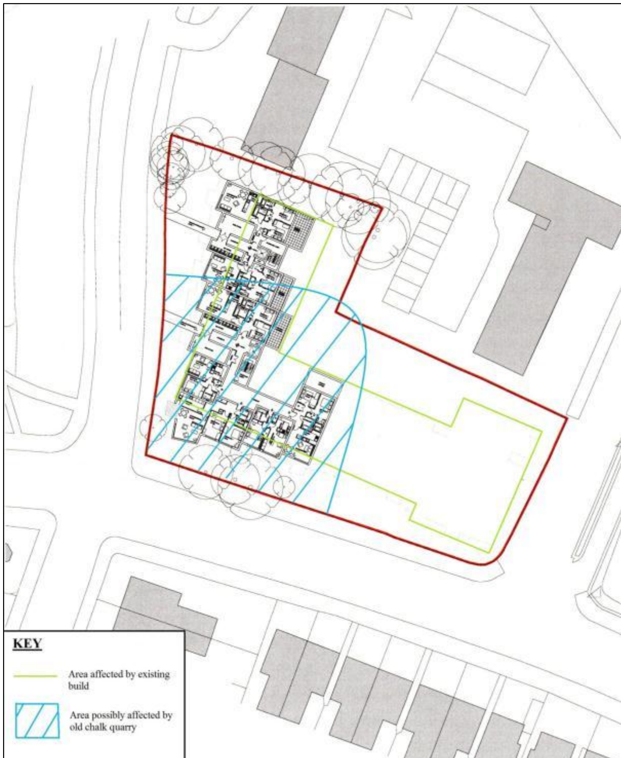
Fig. 13: Park House Hove: Plan of site showing impact of previous developments and old chalk quarry.
