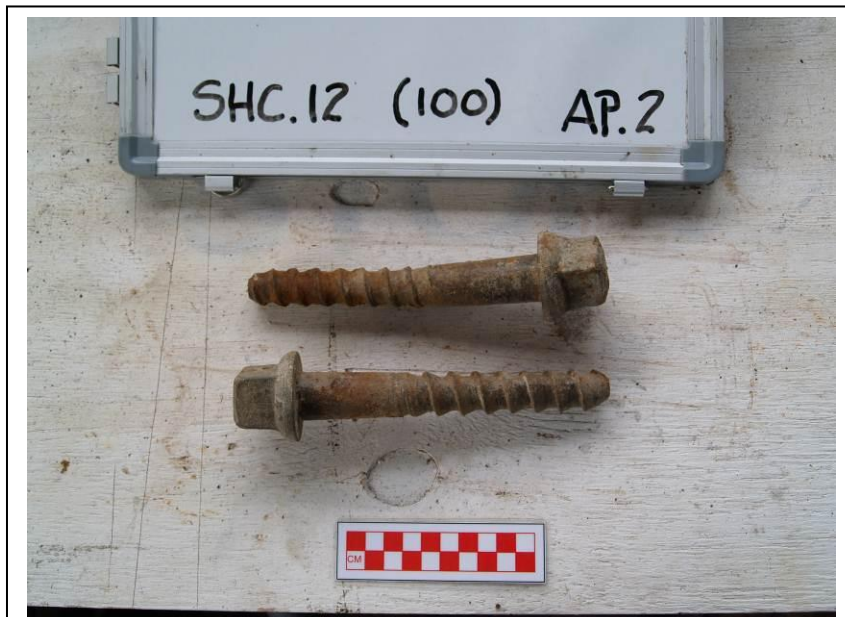
Plate 8: Two Rail Chair Screws found in the Rail Chair shown above
