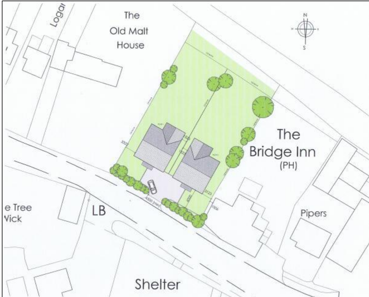
Fig. 10: Former Bridge Inn Car Park, Winchelsea: Preliminary plan of the proposed development (Provided by The Client)
