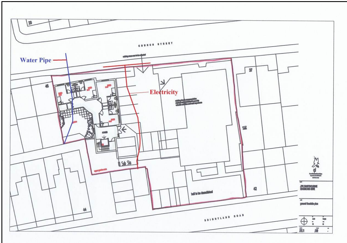
Fig. 15: Edgmond Chapel, Eastbourne: Development Plan, also showing services. (Adapted from architects drawing)
