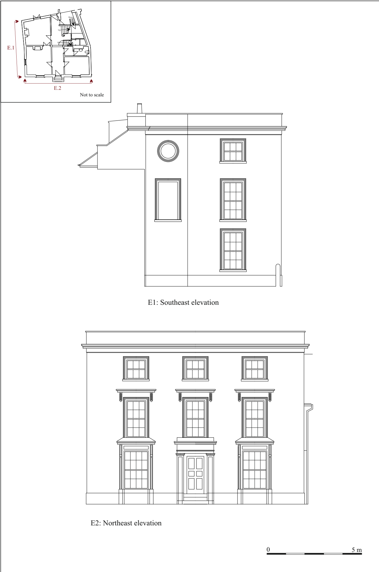
Figure 17: Northeast and southeast external elevations
