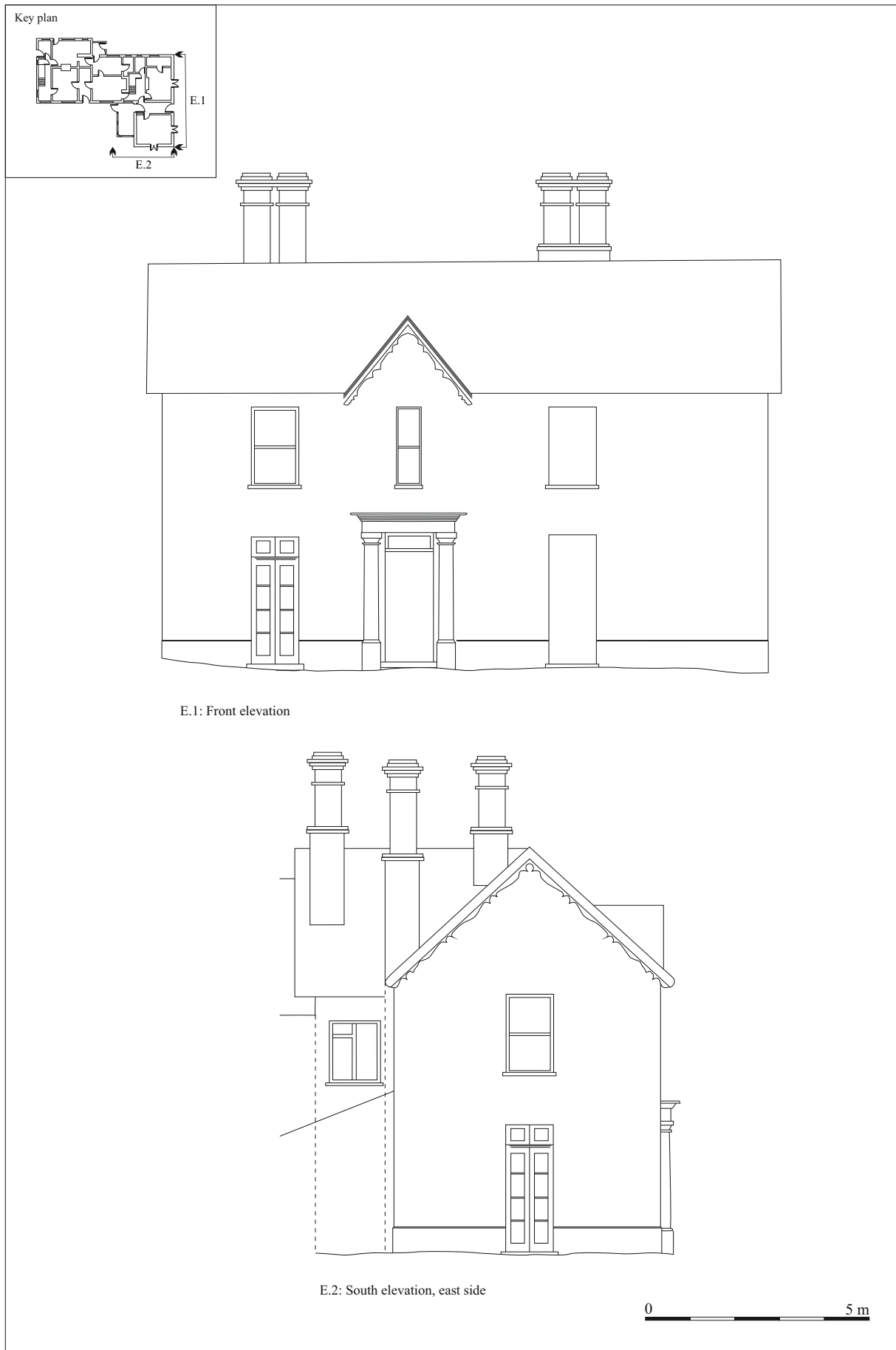
Figure 10: Front and south external elevations
