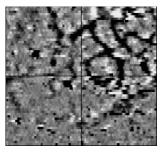
A linear response which is entirely positive in polarity. These are usually related to infilled cut features where the fill material is magnetically enhanced compared to the surrounding matrix. They can be caused by ditches of an archaeological origin, but also former field boundaries, ploughing activity and some may even have a natural origin.
