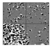
Magnetic debris consists of numerous dipolar responses spread over an area. If the amplitude of response is low (+/-3nT) then the origin is likely to represent general ground disturbance with no clear cause, it may be related to something as simple as an area of dug or mixed earth. A stronger anomaly (+/-250nT) is more indicative of a spread of ferrous debris. Moderately strong anomalies may be the result of a spread of thermoremnant material such as bricks or ash.
