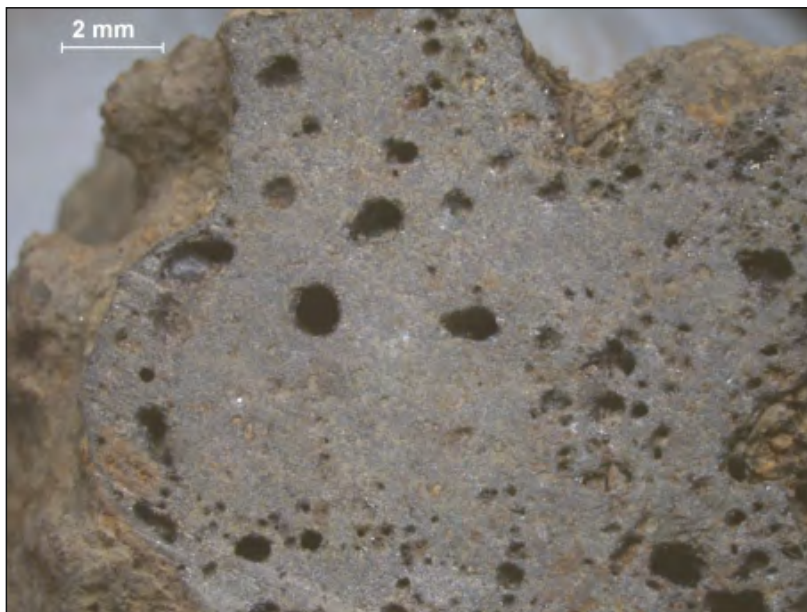
Figure 54. Section through part of one of these PCBs consisting of a dense matrix of mixed iron oxides (partly magnetic) with some porosity (gas holes) and some fine gritty material.
