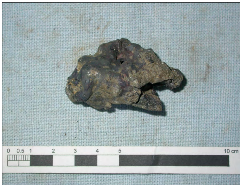
Figure 86. Context (507) (yard metalling). Lightweight, porous (fuel ash) slag formed under intense heat by chemical reaction of some of the hot fuel with the clayey hearth lining.
