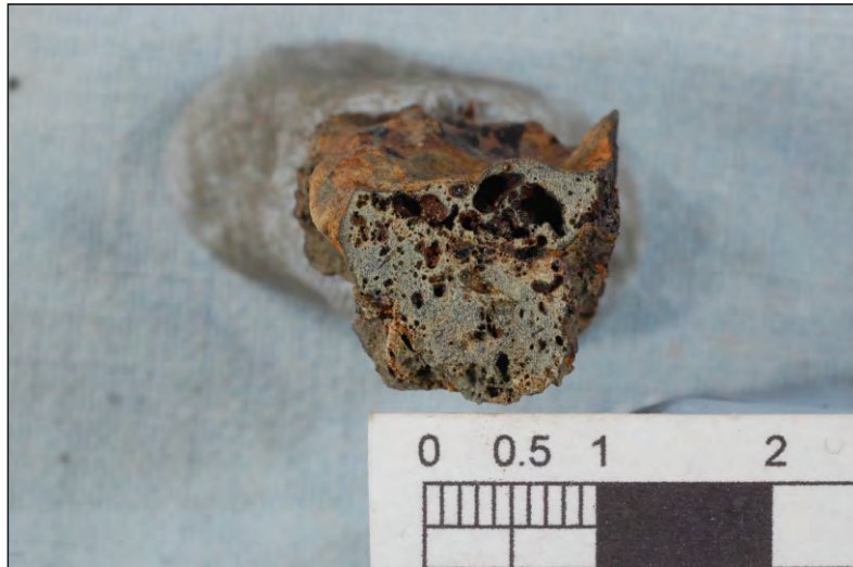
Figure 77. Section cut through a small detached fragment of this SHB/PCB96 showing a mainly fayalitic structure and many voids.
