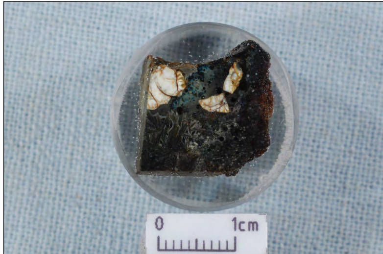
Figure 45. (Context 366) Polished mounted section of a fragment consisting of a mixture of fayalitic iron rich slag (lower left here), fused to which is a fragment of probable fallen hearth wall (above, with larger heat-shattered quartz fragments), both of which are fused to part of the hearth wall lining, the curved line of which is marked by fine pale quartz grit particles, and the reddish inside part of which is also visible (on the right).
