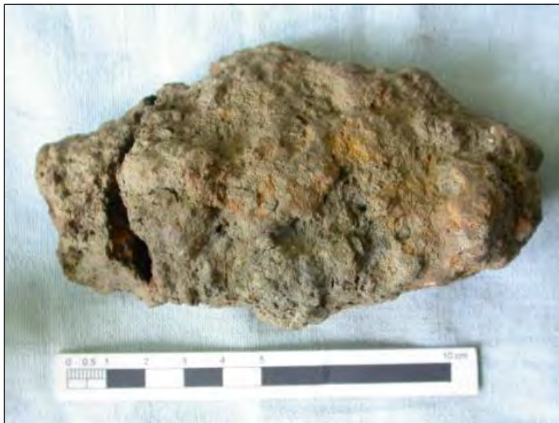
Figure 72. Context (293) of pit 263. A nearly complete, roughly regular PCB/SHB which has formed at the base of a smithing hearth during one campaign of use (? a single day).
