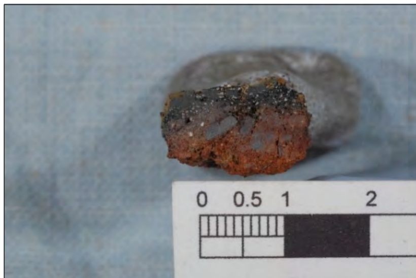
Figure 38. Section of above fragment showing the clayey matrix (grey towards the surface, and oxidised to red inside, below) containing filler material (grog), small fragments of whitish gritty quartz filler plus small (grey) fragments of relatively grit free earlier hearth lining and flakes of hammer-scale, especially noticeable in the more oxidised reddish (inner) zone.
