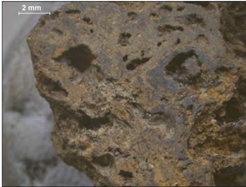
Figure 73. Section from one side of this same PCB/SHB with varying sized holes where slag formed during smithing but did not fully compact.
