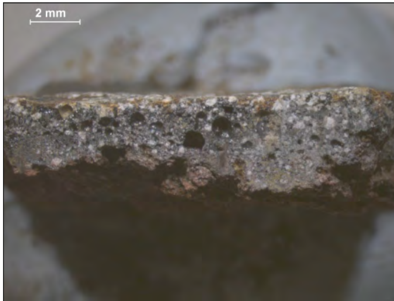
Figure 59. Section through the same fragment of hearth relining showing 8 7 the fine clay dark grey or red matrix containing small fragments of whitish gritty quartz filler, with some flakes of hammer-scale also visible, as are a few small dark grey fragments of crushed re-used hearth wall lining material.
