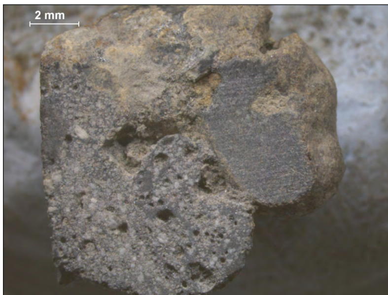
Figure 49. Optical micrograph of the same fragment of hearth (re-)lining in the more vitrified (grey) zone towards the surface of the sample with some partially absorbed heat-shattered quartz fragments plus broken up and dispersed/dissolved fragments of hammer-scale, in a clayey matrix with gas holes voids/voids (image 1.5mm wide).
