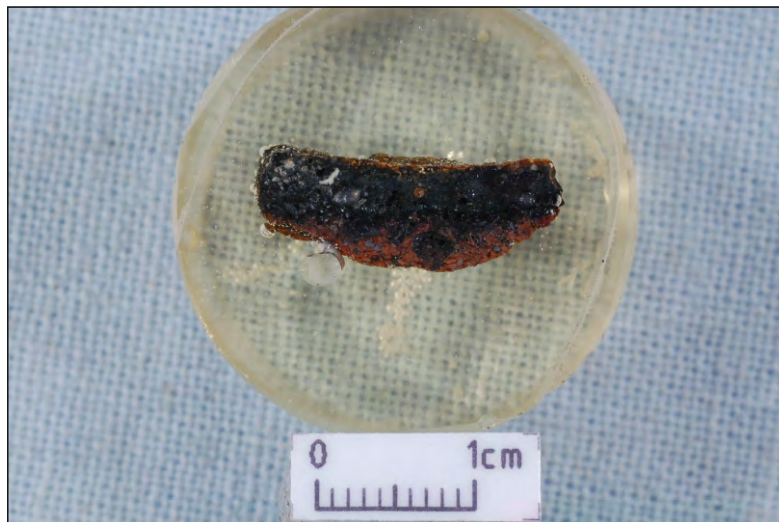
Figure 84. Context (347). Fragment of hearth (re)lining, with hammer-scale flakes visible (as darker flakes) in the fabric on the inner, reddish side (lower part here), although these are largely absent where they have re-dissolved near the outer surface (upper darker part here) where they have dissolved during partial vitrification at the surface.
