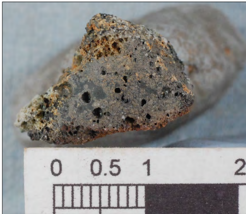
Figure 79. Context (514) from pit 515. Section through a small fragment of fused fuel ash slag/hearth wall, the least altered part of which is the reddish part towards the inner part of the hearth wall, visible here towards the bottom of the fragment.
