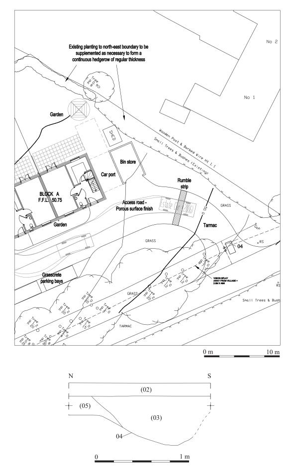
Figure 2. Plan and section of roadside ditch
