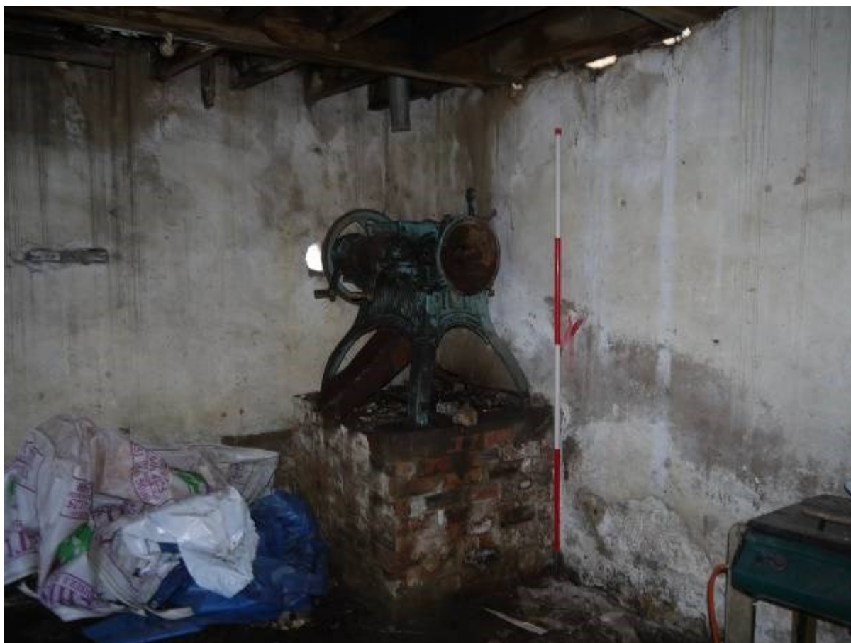
Illustration 29 Bamford Rapid Grinding Rolling Mill in ground floor room of Building B (Phase 1) looking North East (note hole in wall)
